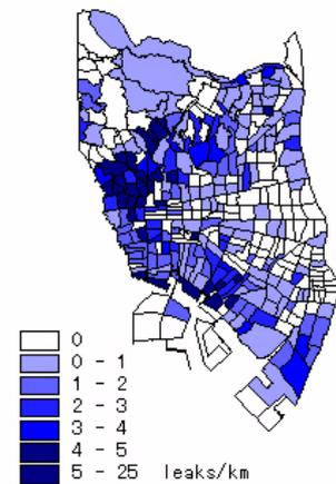
**Fig 6.** Damage of water pipelines.
