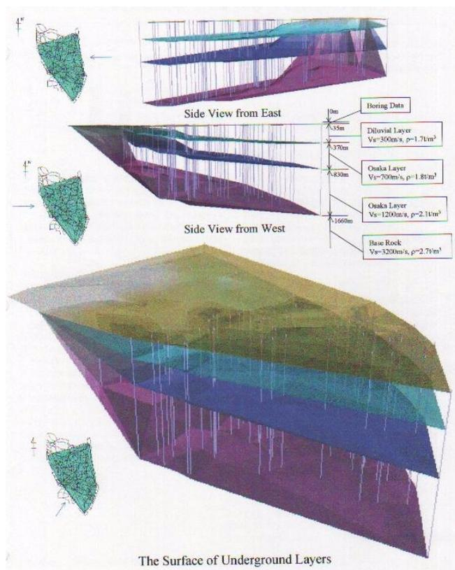
**Fig. 11 Assumed underground layers for ground shaking analysis**
