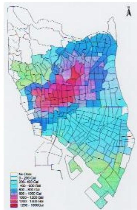
**Fig. 12 The calculated maximum ground acceleration distribution.**
