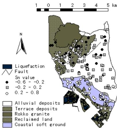
**Fig. 4.** Geological condition and liquefied sites in southern Nishinomiya.
