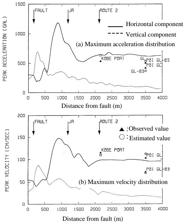
Figure 4: Maximum acceleration and maximum velocity along Sannomiya section
