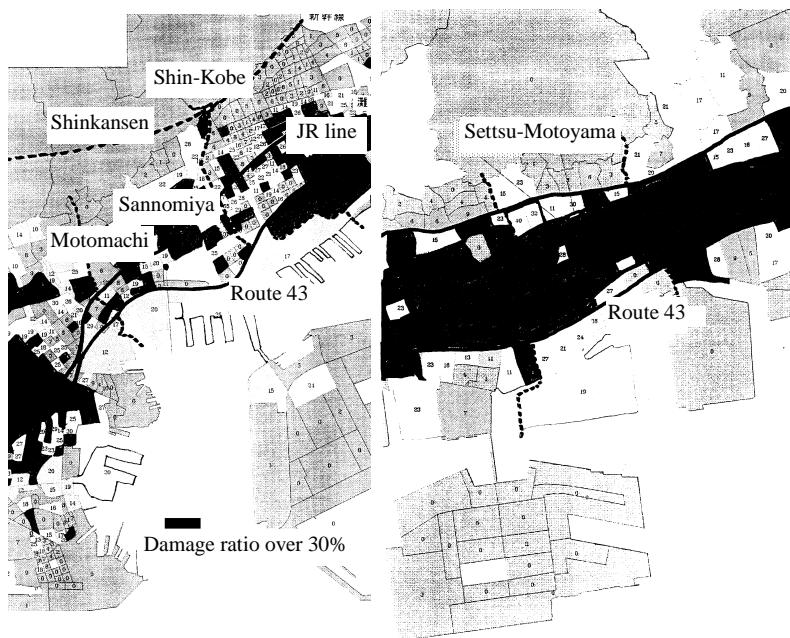
**Figure 1: Damage ratio of low-rise buildings**
