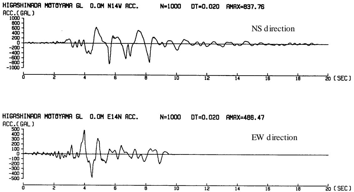
**Figure 6: Computed earthquake waves at Motoyama**
