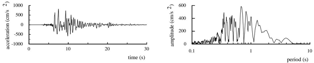
**Figure 4: Kobe –JMA-NS record and their Fourier response spectra.**
