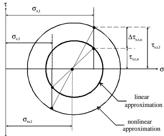
Figure 2: Modified Mohr circle for soil behavior
