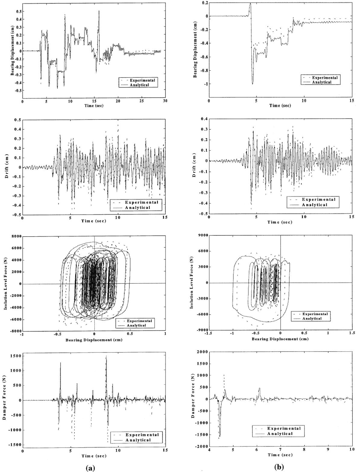
**Figure 3 Experimental and Analytical Results for Base-Isolated Structure with Adaptive Damping (SMC Algorithm) Subjected to (a) 100% of the El Centro Record and (b) 35% of the Rinaldi Record.**
