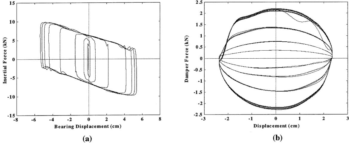
**Figure 2 Force-Displacement Hysteresis Loops: (a) Sliding bearing and (b) Adaptive Fluid Damper.**
