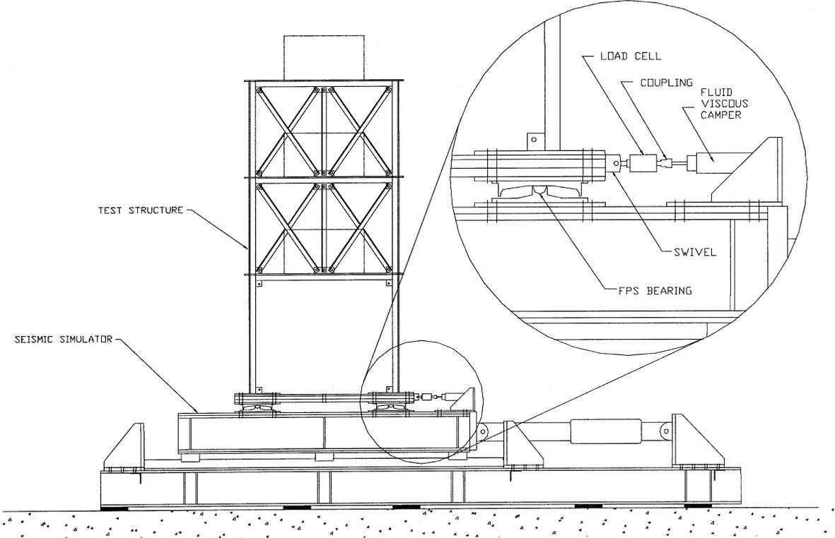
**Figure 1 Test Structure Mounted on Seismic Simulator and Retrofitted with Adaptive Base Isolation System.**
