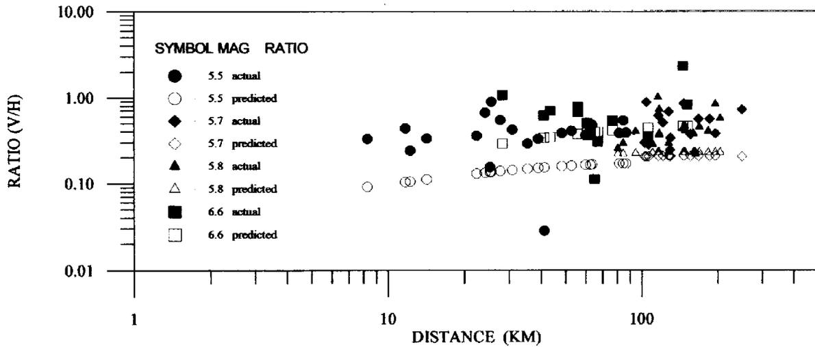
FIG. 5 Comparison of predicted and actual V/H ratio for different magnitudes.
