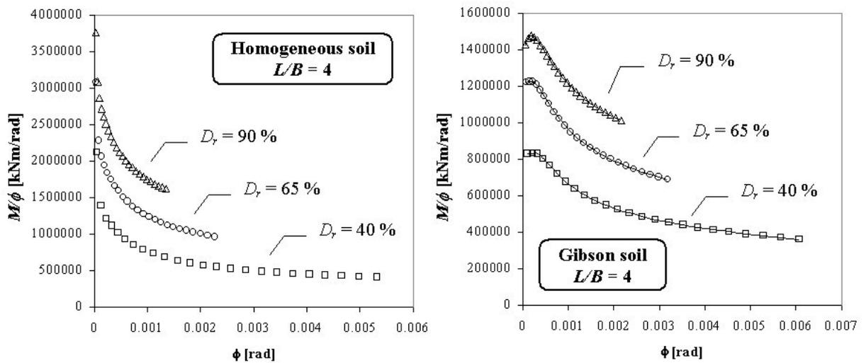
Fig. 5 – Numerical degradation of the rocking stiffness ( $L/B = 4$ )
