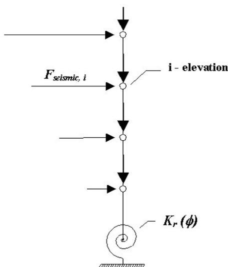
**Fig. 2 – Simplified soil-structure schematization**
