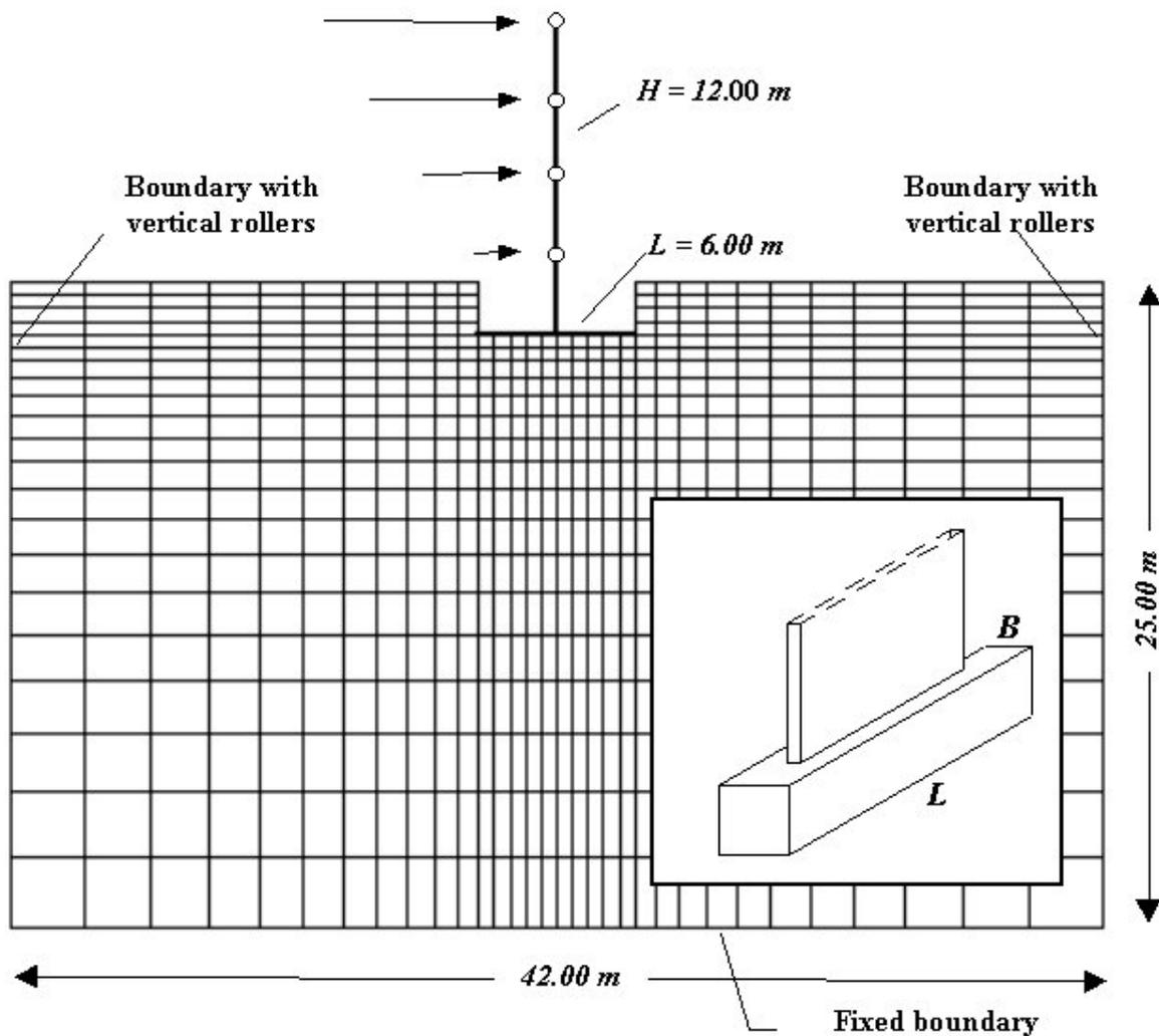
Fig. 1 – Soil-structure system
