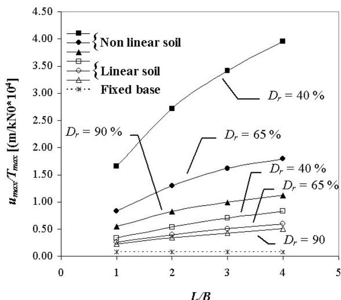
Fig. 6 – The  $u_{max}/T_{max}$  ratio versus the  $L/B$  ratio
