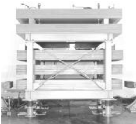
Photo of shaking table test model
