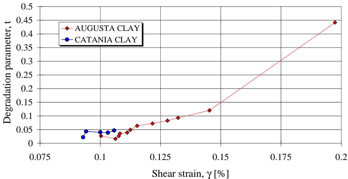
**Figure 5. Degradation parameter  $t$  of Augusta and Catania Clay.**
