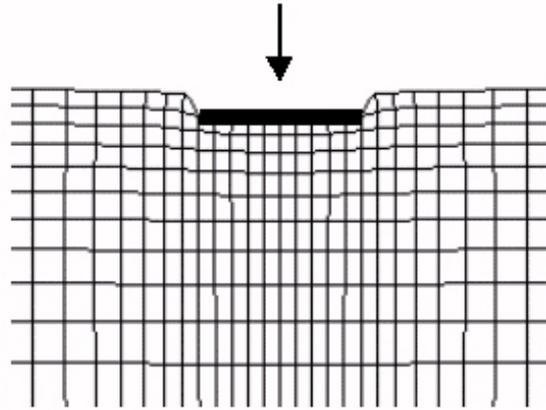
**Fig. 2 – Controlled displacement of the foundation to evaluate vertical stiffness  $K_z$**
