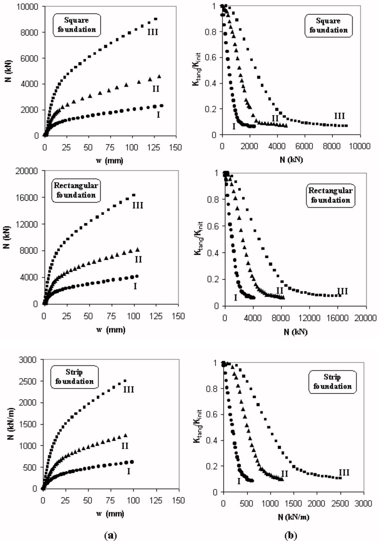
Fig. 5 – Response of the foundations to vertical displacement for different soil conditions
