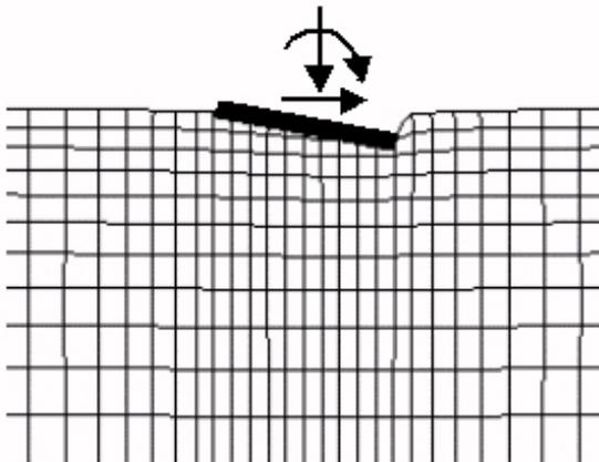
**Fig. 3 – Controlled displacement of the foundation to evaluate rocking stiffness  $K_{\phi,x}$  in absence of up-lifting, settling and swaying**
