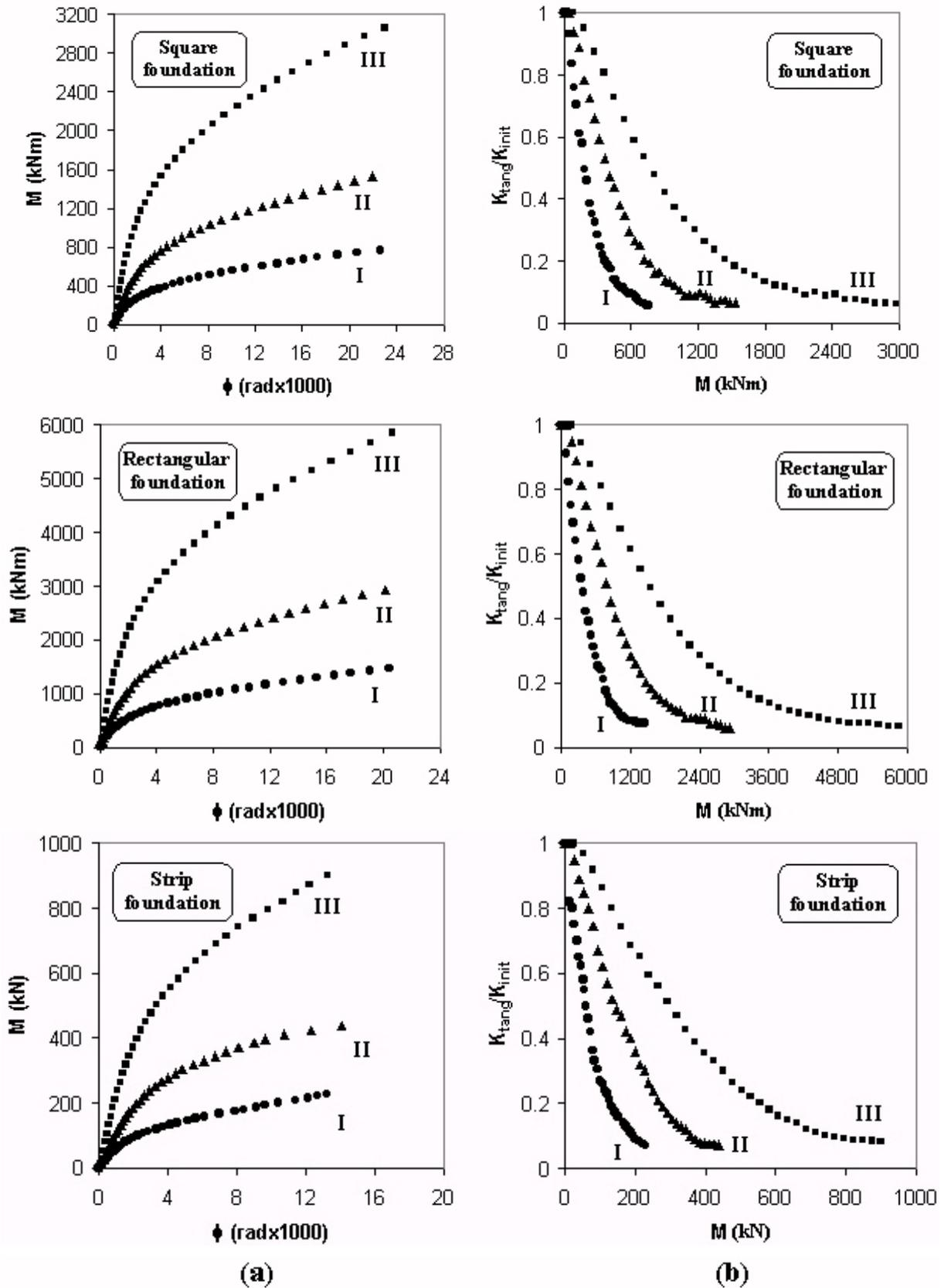
Fig. 6 – Response of the foundations to rocking displacement for different soil conditions
