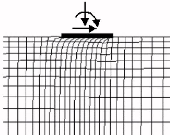
**Fig. 4 – Controlled displacement of the foundation to evaluate swaying stiffness  $K_y$  in absence of rotation, settlement and up-lift**
