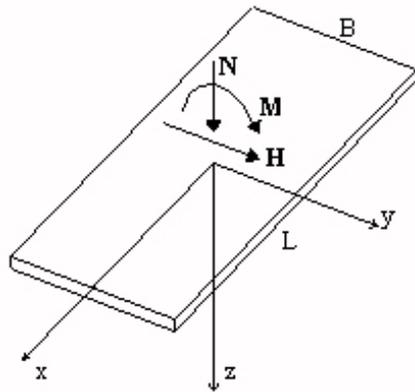
**Fig. 1 – Rigid foundation geometry and selected reference system**
