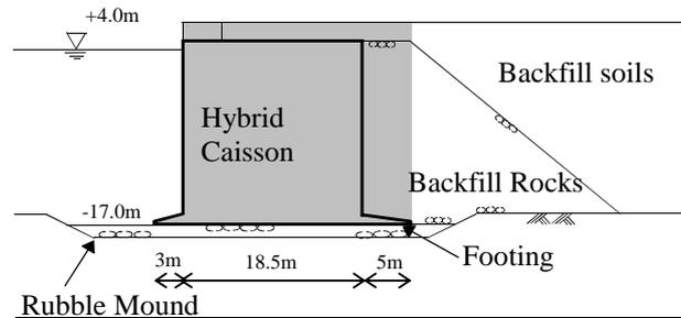
**Fig.2: The prototype of the Hybrid Caisson-type quay wall**
