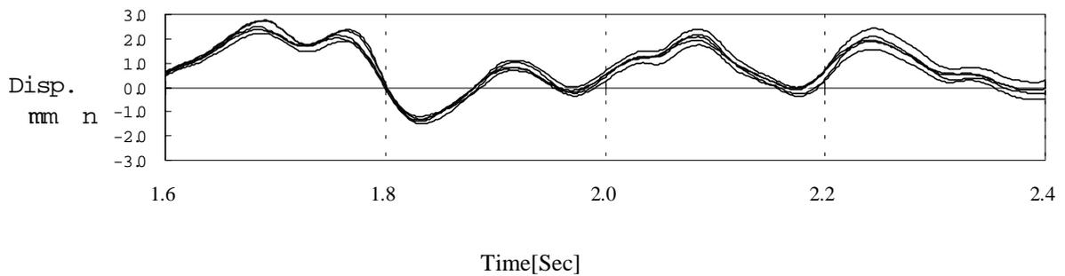
**Fig.7: Displacement time histories obtained by integrating accelerations (AH20, AH5- AH8, AH22)**
