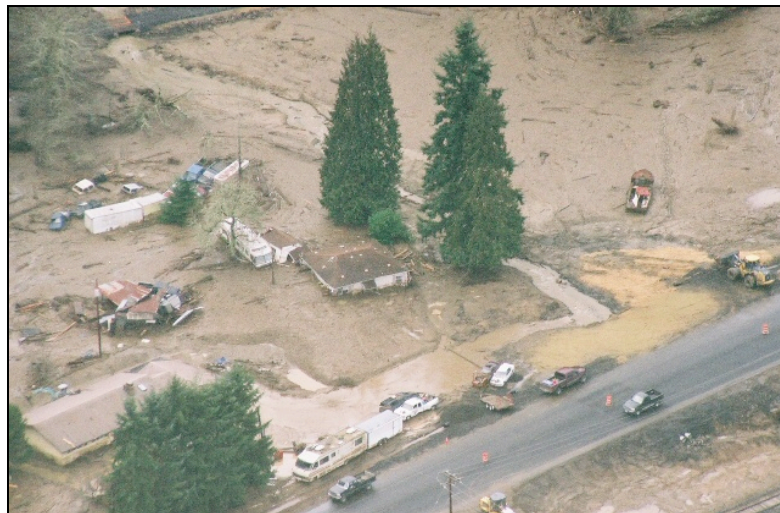
Figure 2. Debris Flow Fan that Inundated a Community and Lifelines
