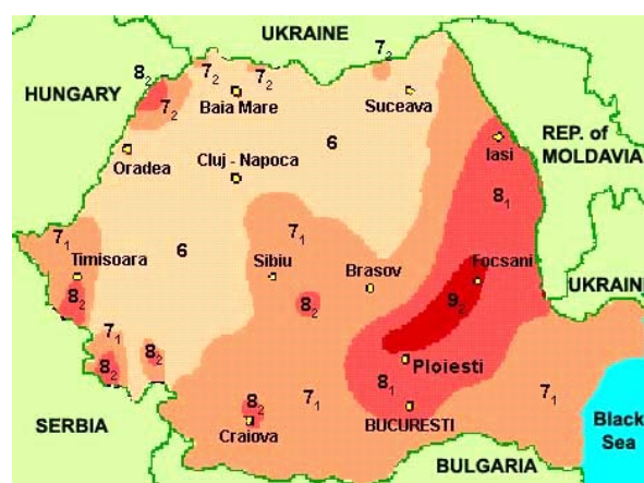
Figure 1. Recent strong earthquakes and the seismic zonation map (in terms of intensities) of Romania
