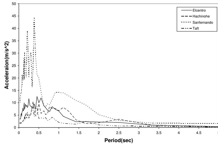
Figure 5. Response spectra of different earthquakes with damping ratio of  $\xi = 2\%$
