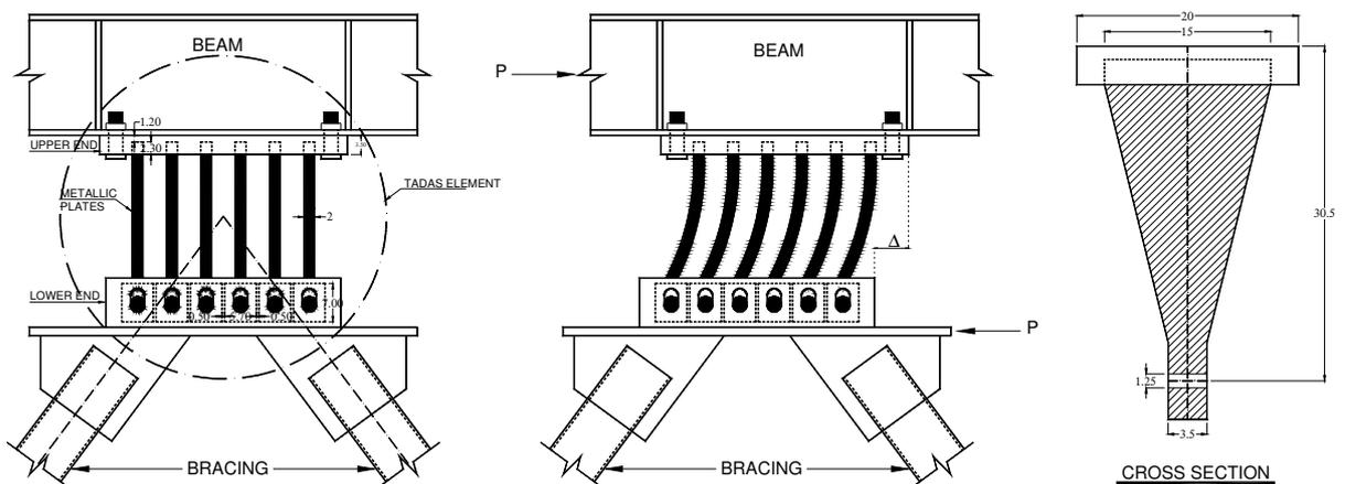
Figure 2. The behavior of TADAS damper during earthquake (all dimensions in centimeter)
