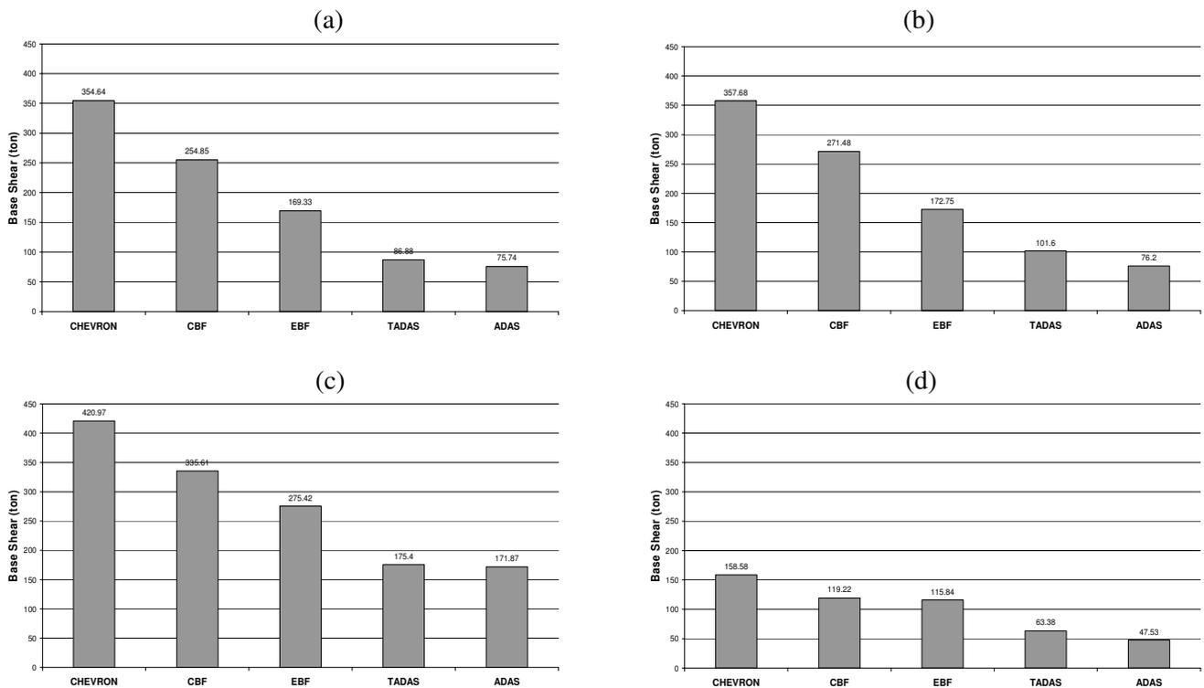
Figure 6. Maximum induced base shear force of different systems
