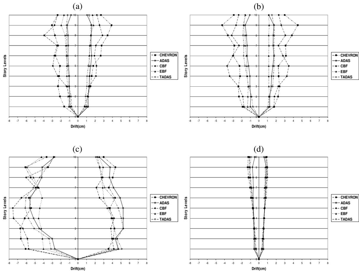
Figure 7. Maximum drift of different systems; a) Elcentro, b) Hachinohe, c) San Fernando, d) Taft
