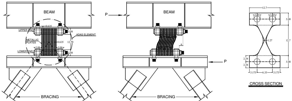
Figure 1. The behavior of ADAS damper during earthquake (all dimensions in centimeter)
