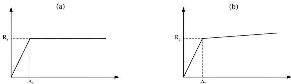
Figure 3. Proposed load-deformation for ADAS & TADAS dampers
