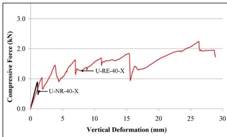
Figure 5 Force vs. vertical deformation for unburned brick (adobe) masonry wallette
