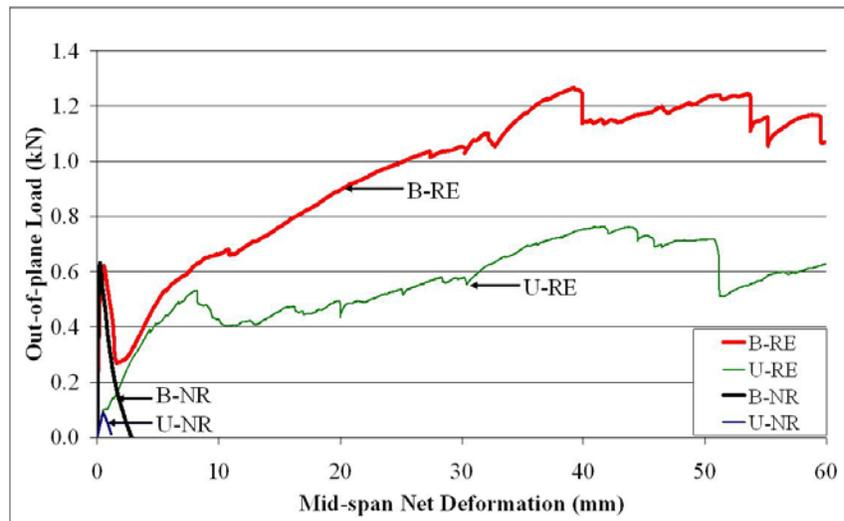
Figure 10 Out-of-plane load variation in terms of net vertical deformation
