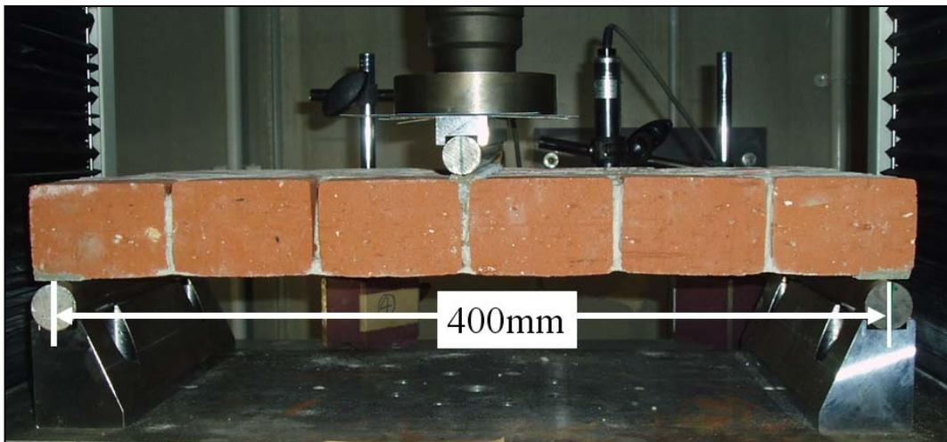
Figure 8 Out-of-plane test setup
