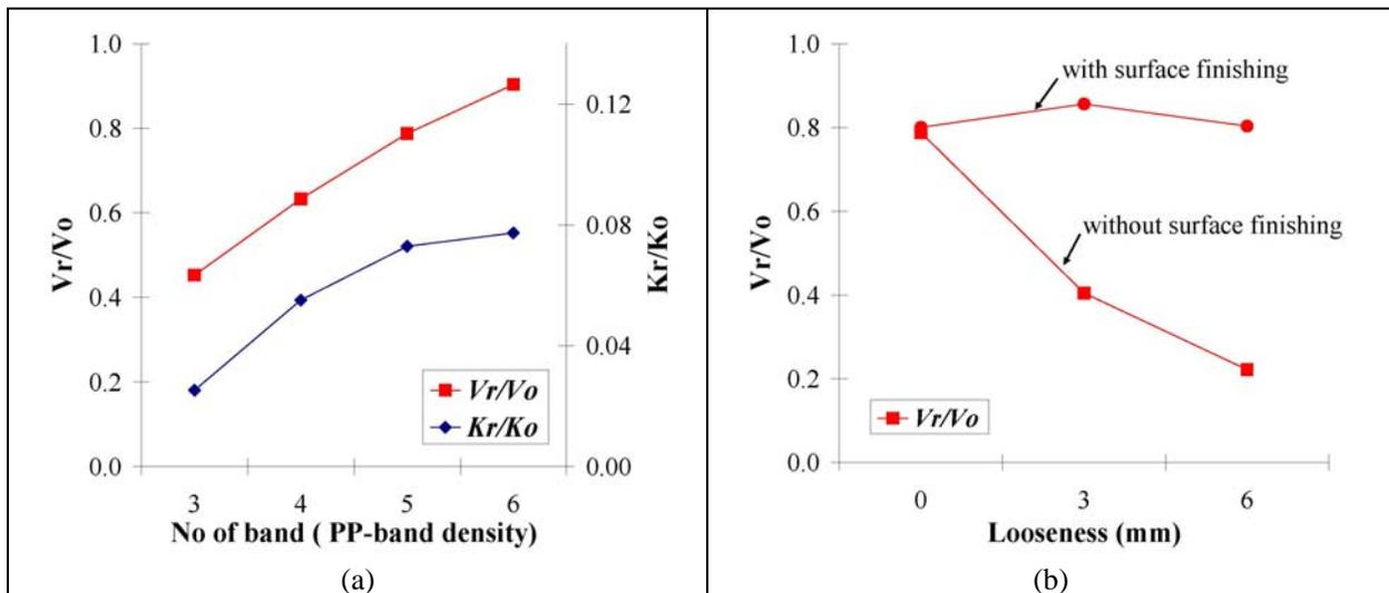
Figure 7 (a) Effect of PP-band density (b) Effect of looseness between wallette and PP-band mesh
