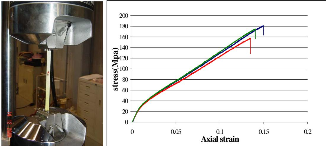
Figure 1 Tensile test setup (left) behavior of PP-band under tension (right)
