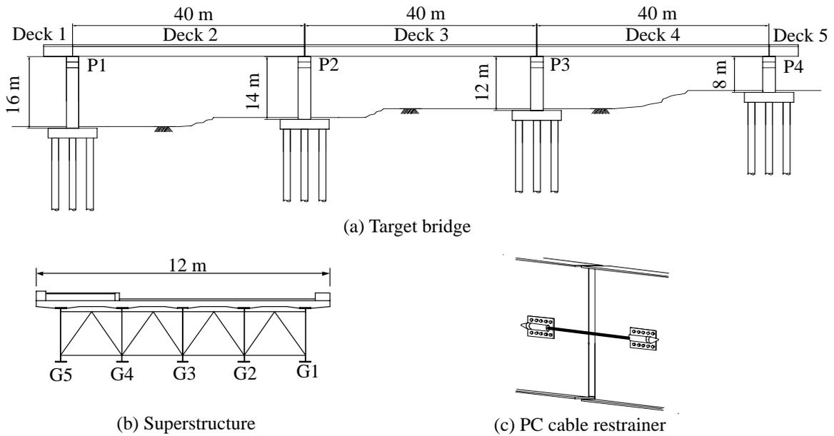
Figure 1 Target Bridge and Restraints
