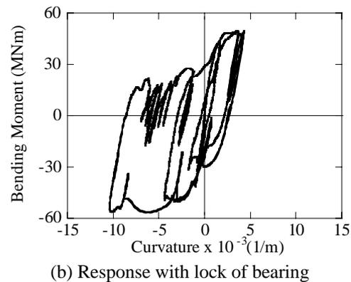
Figure 13 Moment vs. Curvature Hystereses of P2 at the Plastic Hinge in the Longitudinal Direction
