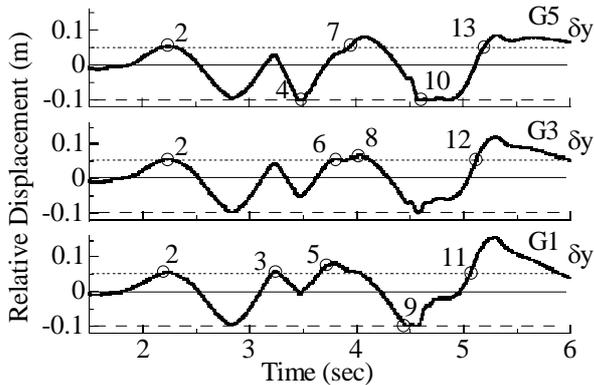
(b) Relative displacement between decks ( $\Delta u_{23}$ )
