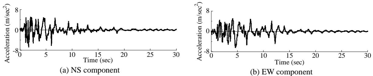
Figure 4 JR Takatori Station Record during 1995 Kobe Earthquake
