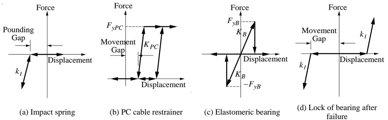
Figure 3 Idealization of Pounding, Restraints, Elastomeric Bearing and Lock of a Bearing after Failure
