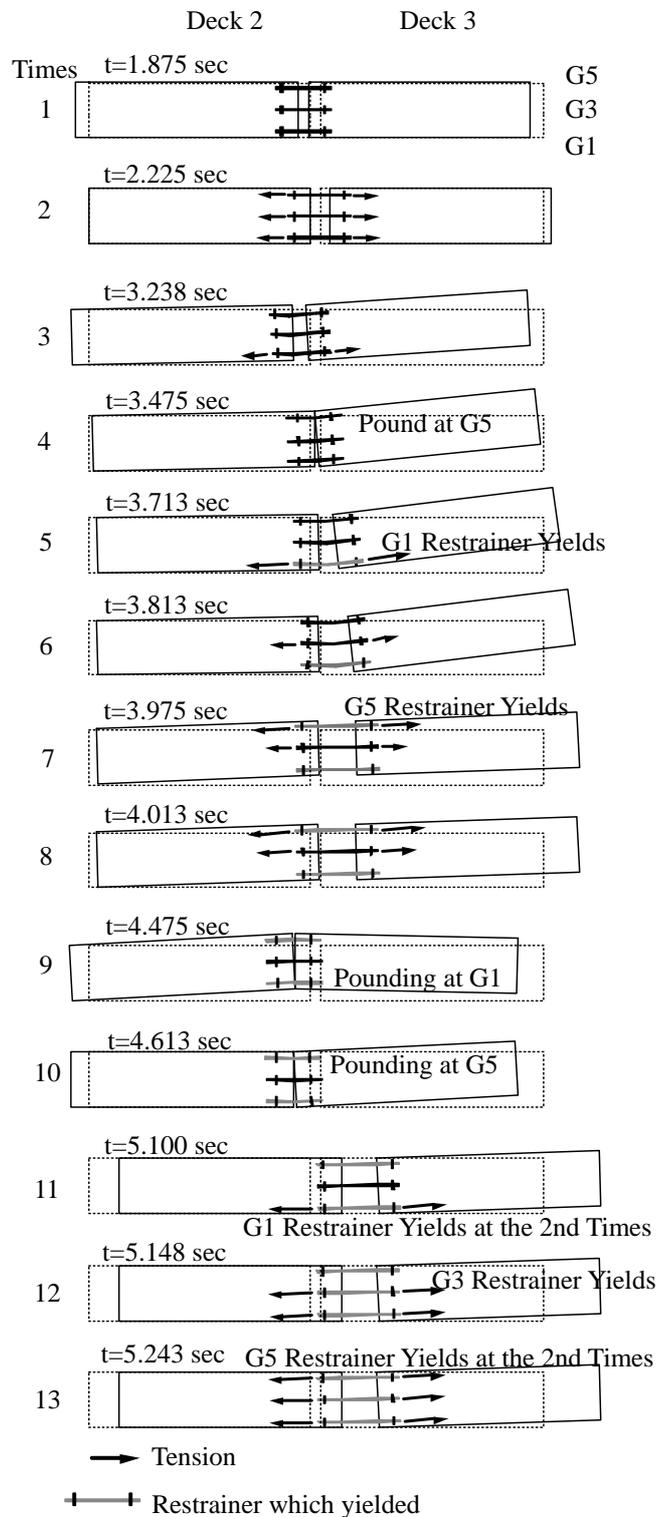
Figure 7 Deck Response with Poundings and Yielding of Restrainers
