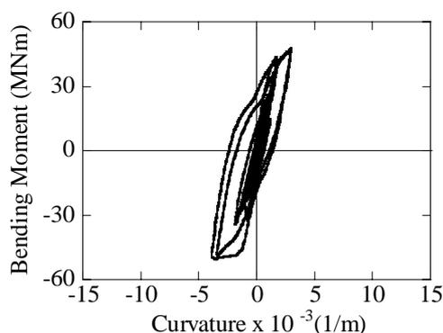
Figure 8 Moment vs. Curvature Hystereses of P2 at the Plastic Hinge in the Longitudinal Direction
