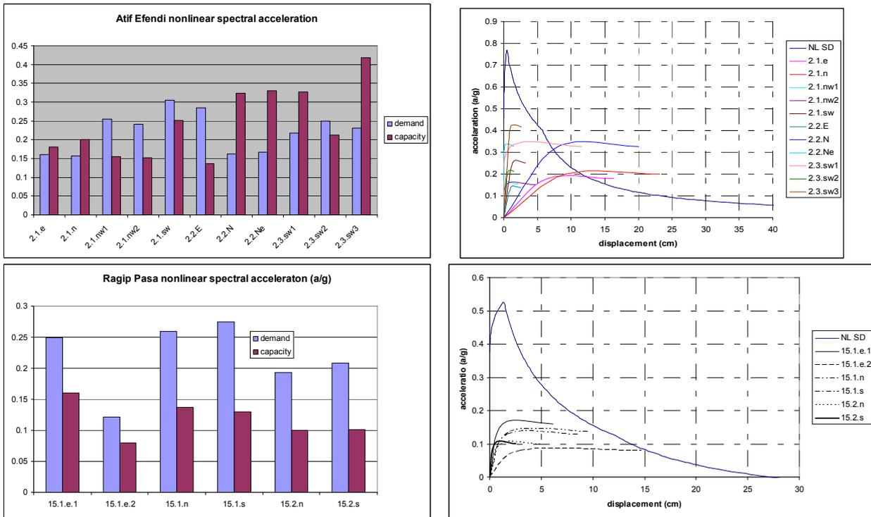
Figure 2 Comparison of capacity and demand for each of the assessed elevations in terms of acceleration and in terms of equivalent push over analysis performance points.
