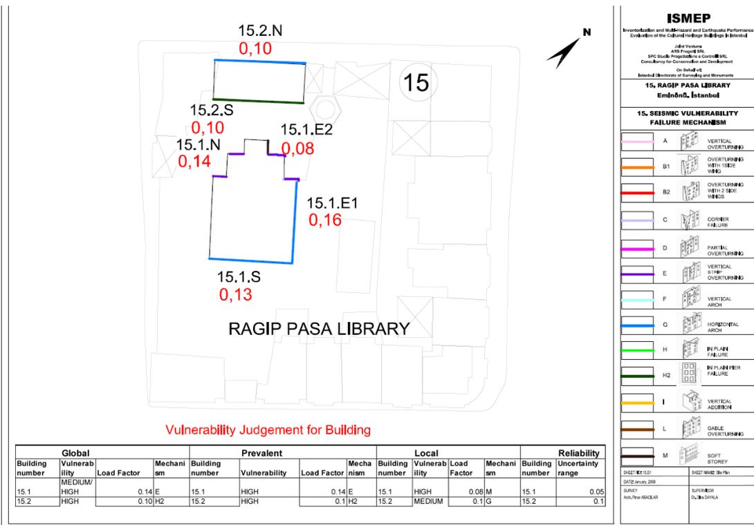
Figure 1 Mapping of load factor mechanism of collapse and overall vulnerability judgement for each compound.
