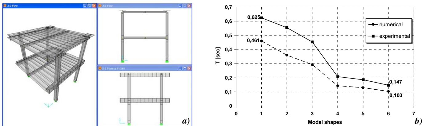
Figure 3 FEM model of the bare structure (a) and comparison in terms of modal frequencies (b)
