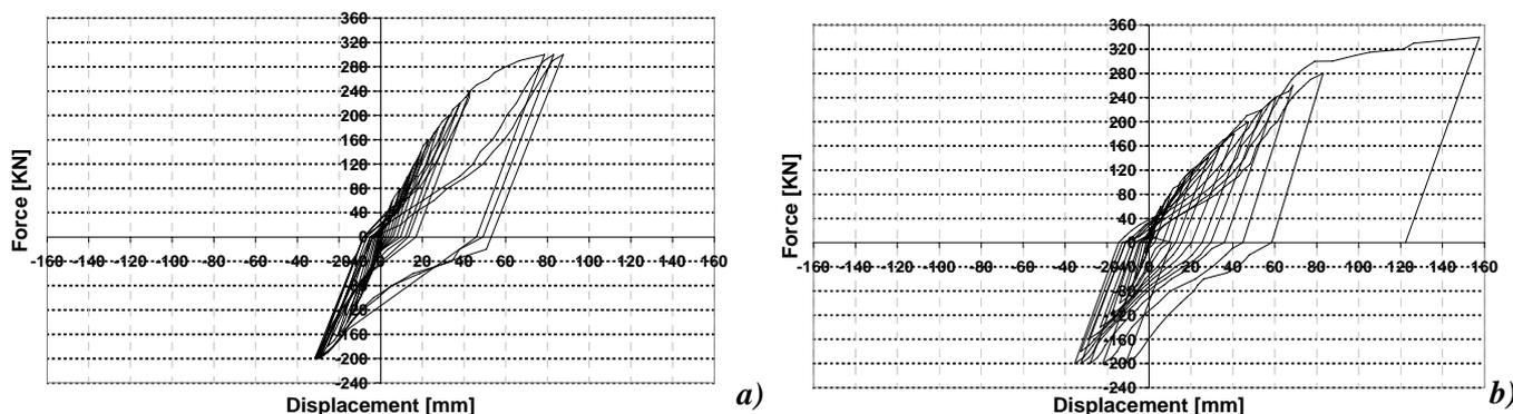
Figure 8 Lateral response of the RC structure retrofitted with steel (a) and pure aluminium (b) shear panels
