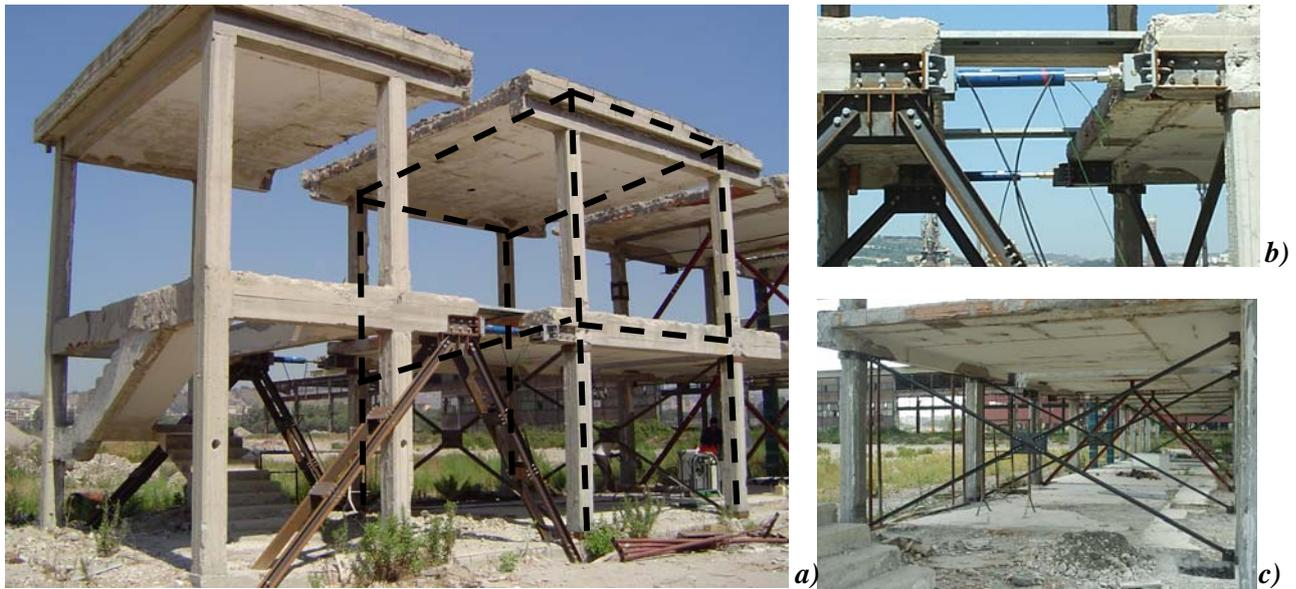
Figure 1 The analyzed structure (a), the hydraulic jacks (b) and the X-bracings system (c)
