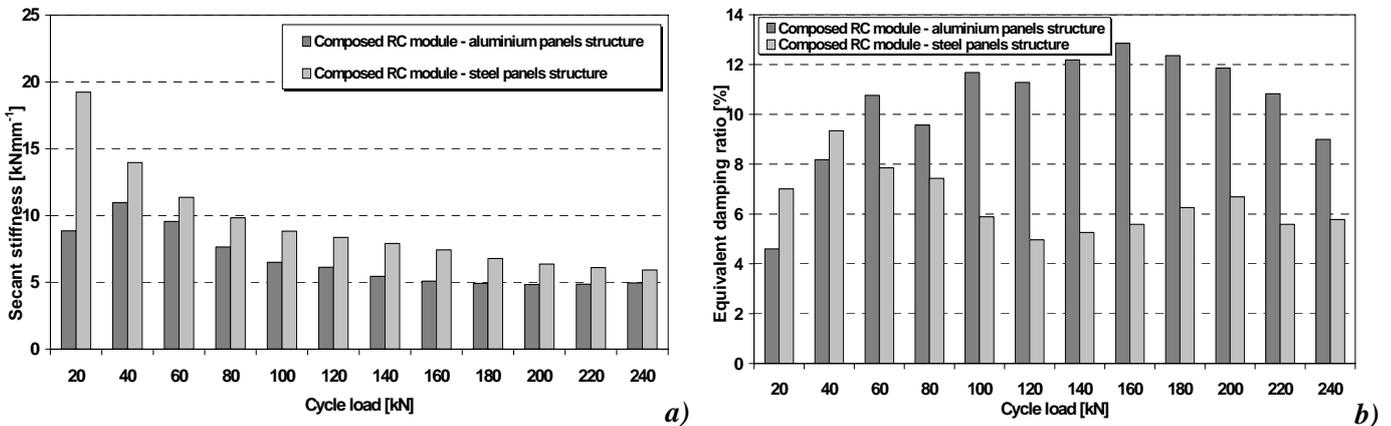
Figure 11 Comparison of results in terms of secant stiffness (a) and equivalent viscous damping ratio (b)
