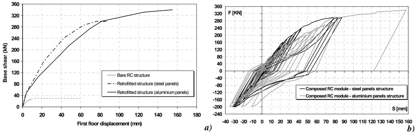
Figure 10 Comparison of results in terms of envelope curves (a) and hysteresis cycles (b)
