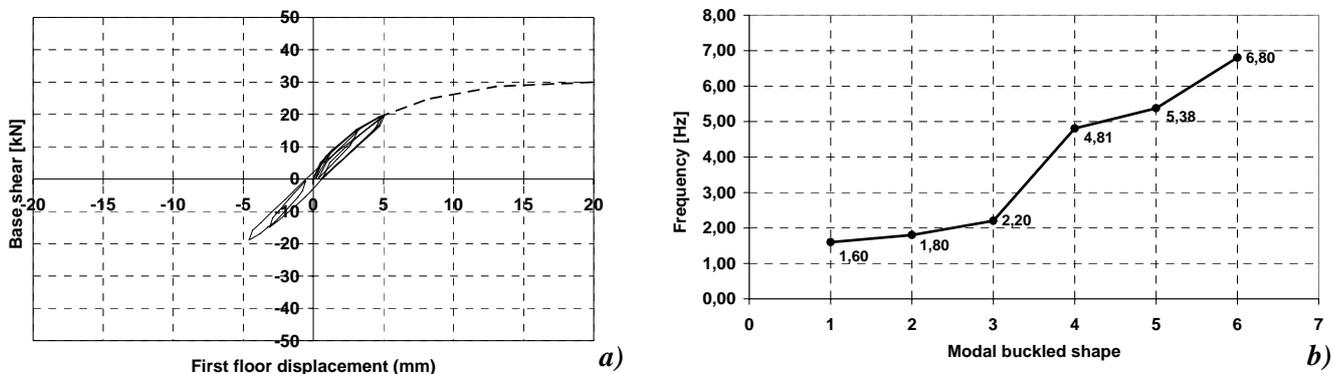
Figure 2 The bare RC structure: response to lateral loads (a) and modal frequencies (b)
