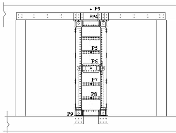
Figure 7 Measurement transducers used in the experimental tests
