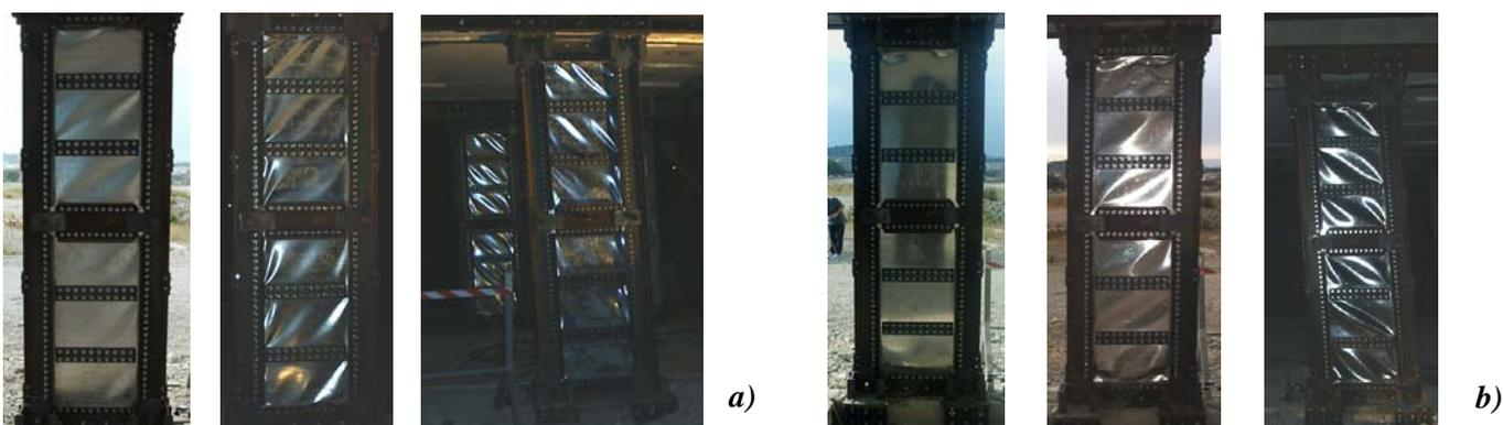
Figure 9 Development of the tension field mechanism into steel (a) and pure aluminium (b) shear panels
