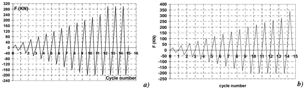
Figure 6 Loading protocol used in the test for steel (a) and aluminium (b) shear panels
