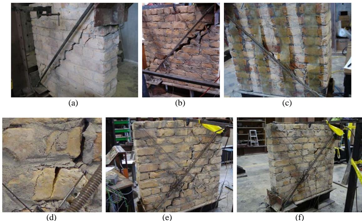
Figure 5 Test wallette failures: (a) DS-0; (b) DSG-3; (c) DSG-3 FRP debonding; (d) DSG-4, crack passing through brick and masonry joint; (e) DGS-4; and (f) DSG-5.
