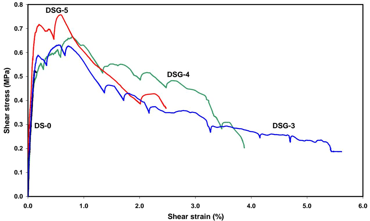
Figure 4 Shear stress versus shear strain curves for the test wallettes
