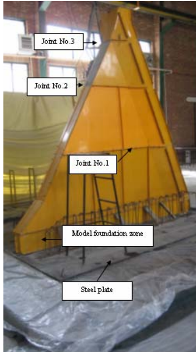
Figure 2: Layout of construction joints
