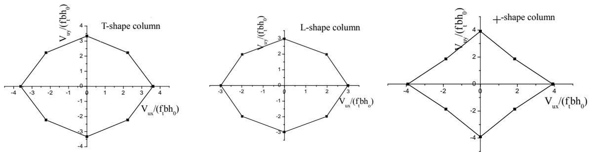
Figure 3 Relationship between shear-bearing capacity and loading direction for SRC special-shaped columns
