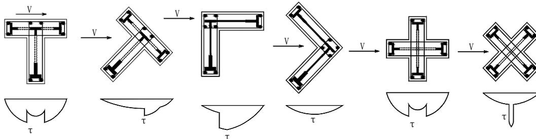
Figure 4 Shear stress distributions in different loading direction of SRC special-shaped columns
