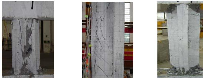
(a) shear-diagonal compression failure (b) shear-bond failure (c) flexural failure
