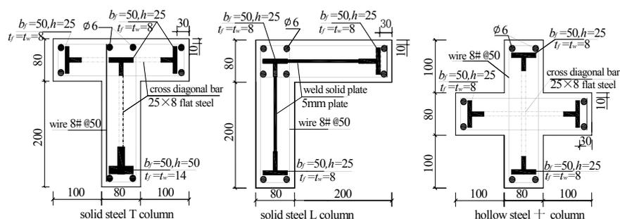
Figure 1 Geometry and steel details of specimens
