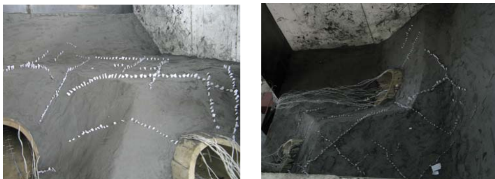
Fig. 7 Crack distribution on damaged soil after final excitation
