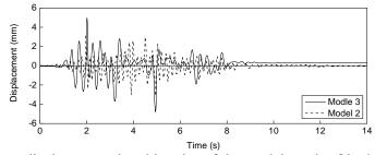
Figure 7 1st-story displacement time histories of the models under Qian'an earthquake
