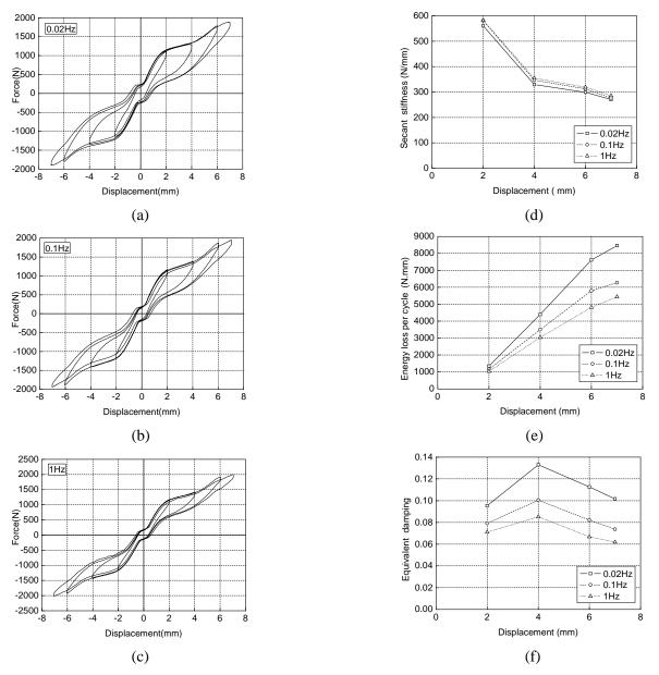
Figure 4 Mechanical behaviors of the RDD at different displacement amplitudes and frequencies
