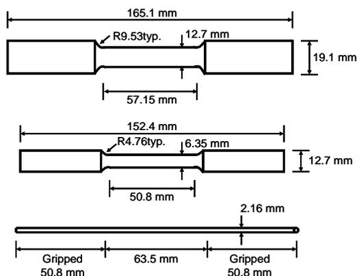
Figure 2 Drawings of the bar and wire specimens.
