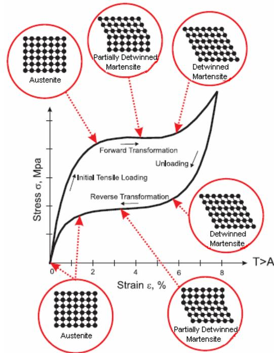
Figure 1 Typical stress-strain curve for a superelastic shape memory alloy cycled in tension.
