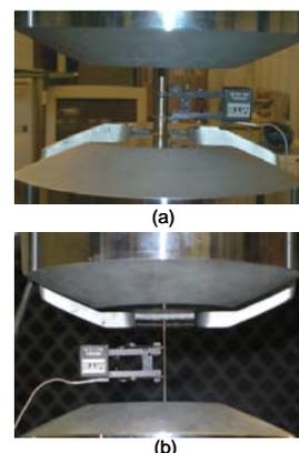
Figure 3 Test setup for the (a) bars and (b) wires.
