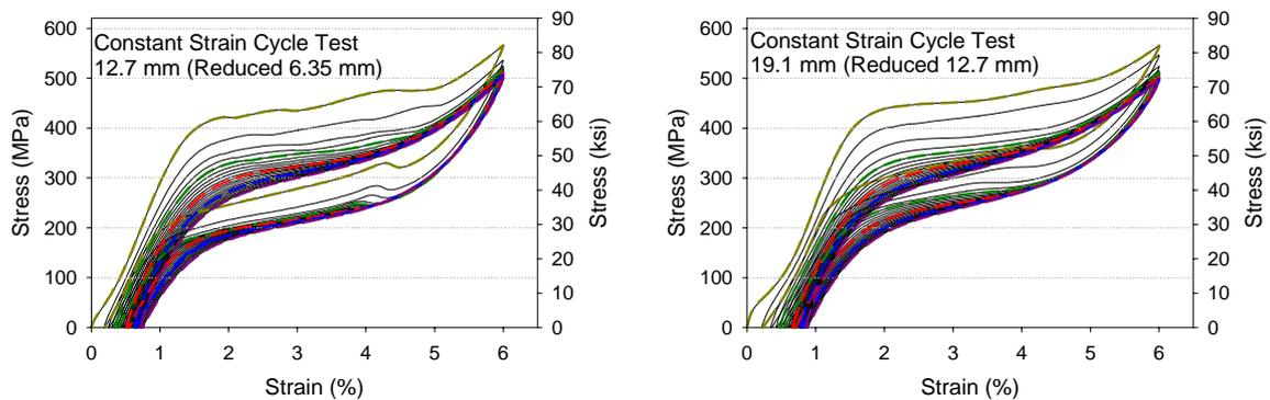
Figure 4 Constant strain cycle test stress-strain plots for a representative 12.7 mm and 19.1 mm diameter bar (dashed lines represent label the 1<sup>st</sup>, 5<sup>th</sup>, 10<sup>th</sup>, 15<sup>th</sup>, and 20<sup>th</sup> cycles).
