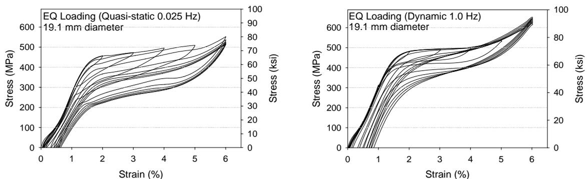
Figure 6 Earthquake-type loading test stress-strain plots for representative 19.1 mm diameter bars tested at 0.025 Hz (quasi-static) and 1.0Hz (dynamic).
