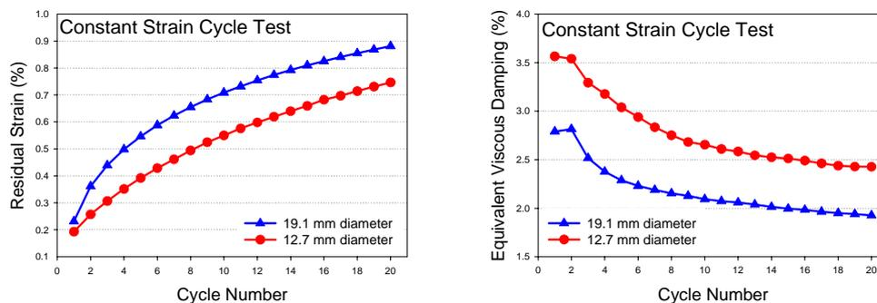
Figure 5 Residual strain and equivalent viscous damping properties with respect to cycle number.
