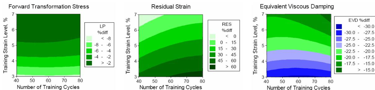
Figure 8 Response surface study results with respect to mechanical training factors.
