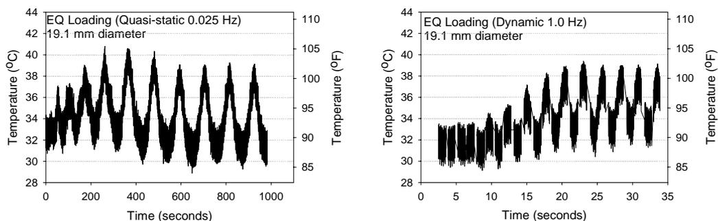
Figure 7 Surface temperature fluctuation during cycling of representative 19.1 mm diameter bars.
