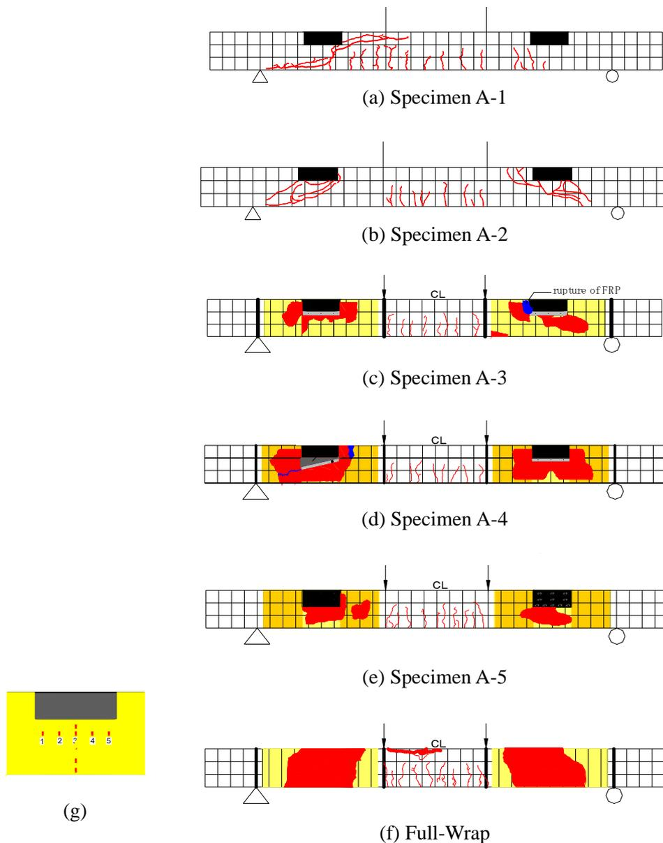
Figure 7 Condition of specimens at the ultimate state (a-f) and location of strain gages in U-wrap.
