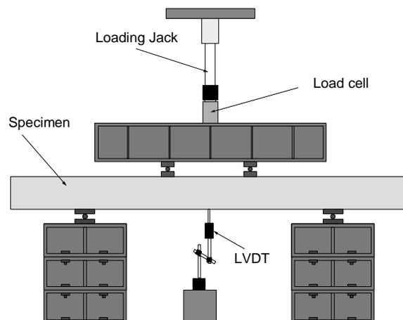
Figure 5 Test setup.
