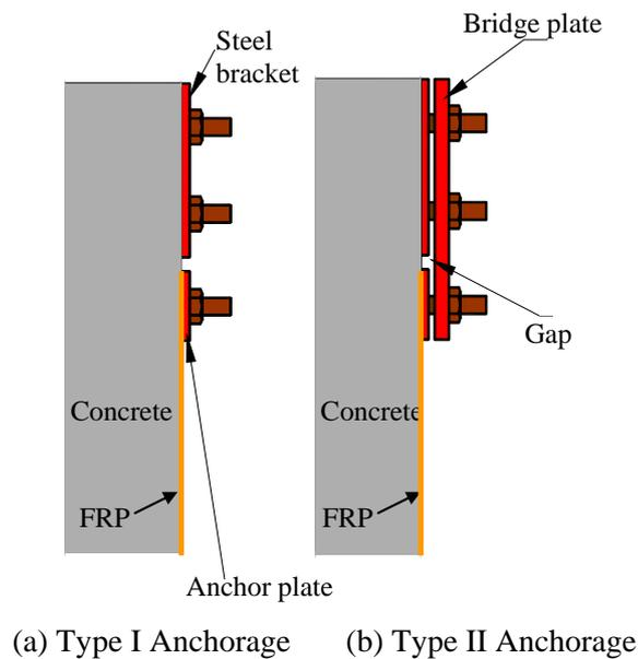
Figure 4 Mechanical anchorage.
