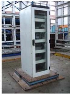
Figure 3 Motion sensitive equipment with the SDI-BPS isolators
