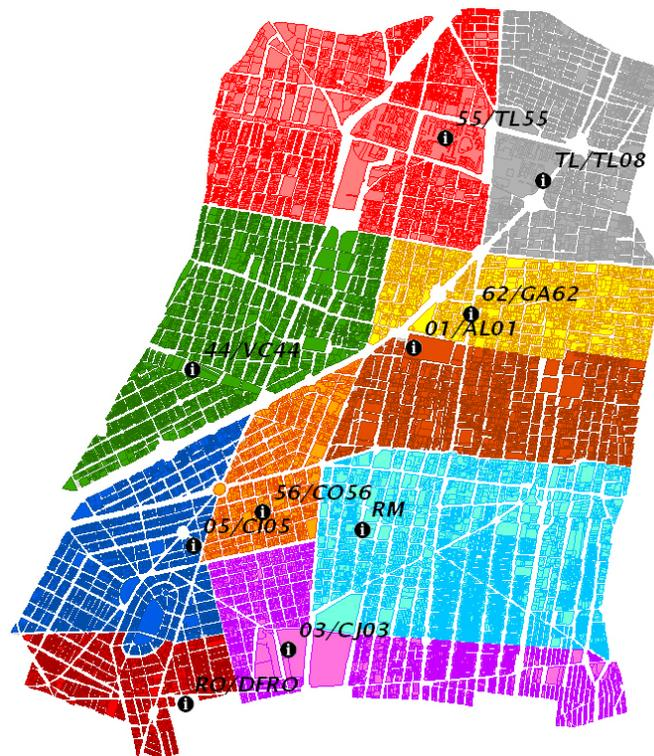
Figure 2 Central part of Mexico City where colors show the regions where a specific accelerogram is going to be used to compute the structural response of all buildings within each region. The selected accelerometric stations are shown for each region
