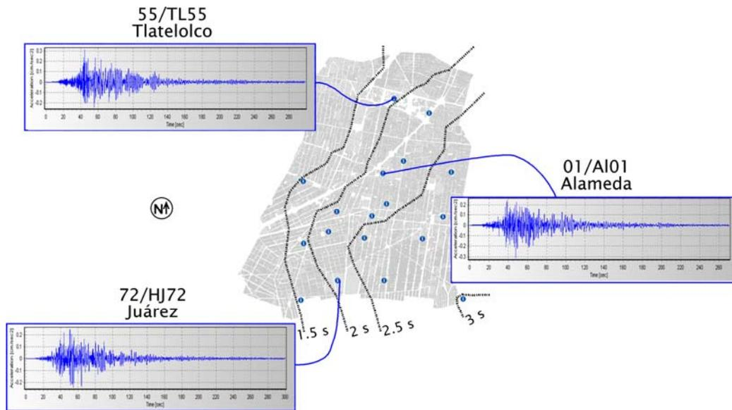
Figure 1 Central part of Mexico City with lines of equal dominant period and accelerometric records that we have considered as representative for determined regions. As examples, records from the 19/04/99 earthquake are shown for stations 01, 55 and 72
