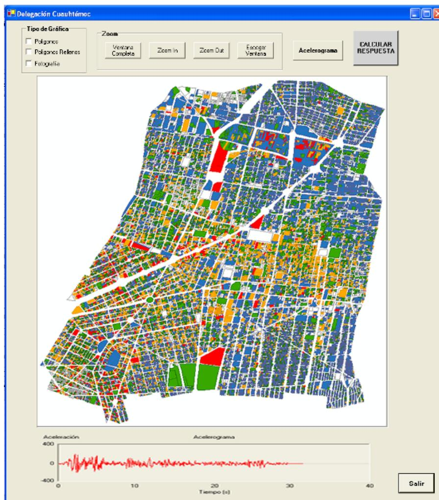
Figure 3 Example of the software to estimate maps of losses. It shows losses for the accelerogram drawn at the bottom of the figure
