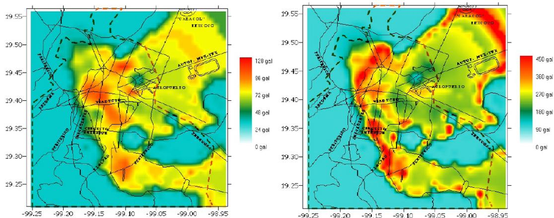
Figure 6 Shake maps for Mexico City for a given scenario (Alcántara and Ordaz, 2008) for ground motion (left) and for a structural period of  $T=2.0$  sec (right)
