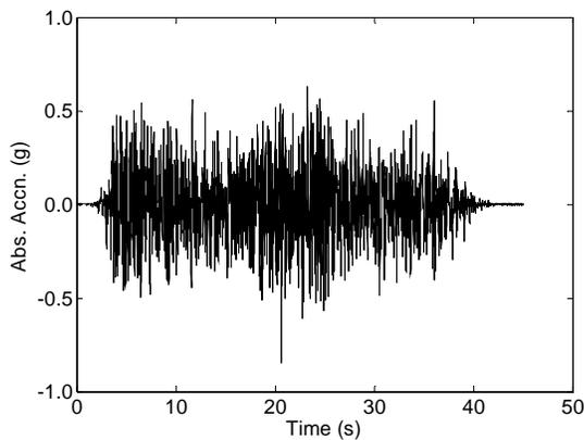
c) Analytical roof acceleration response (fixed model)
