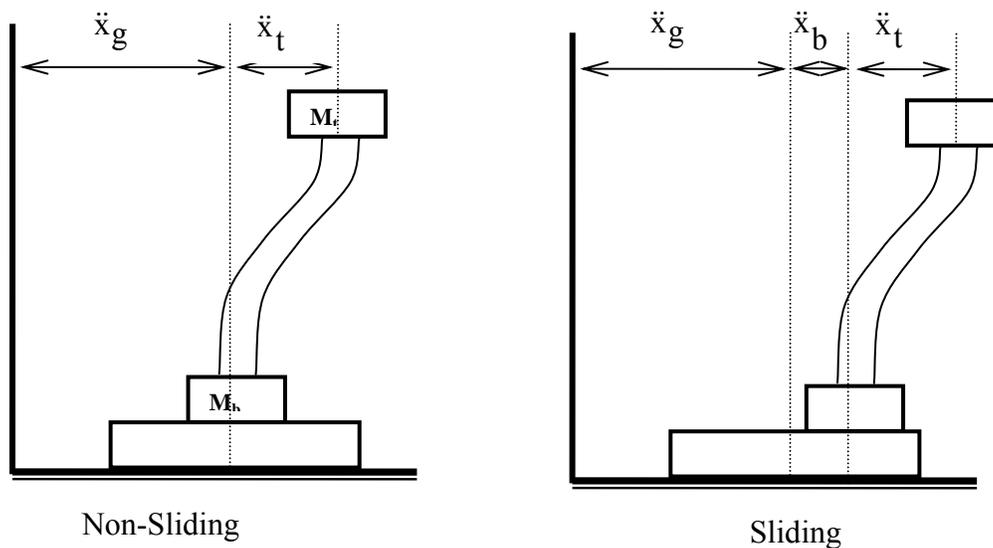
Figure 1: Schematic diagram for non-sliding and sliding system
