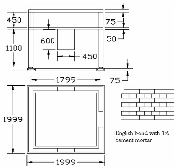
Figure 5: Plan and elevation (all dimensions in mm)
