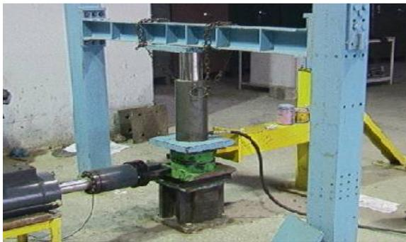
Figure 2: Experimental set up for friction test with shear box
