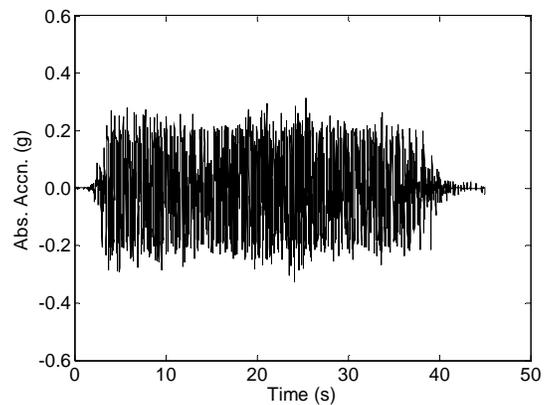
d) Analytical roof acceleration response (sliding model)
