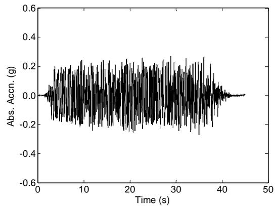
b) Experimental roof acceleration responses (Filtered)
