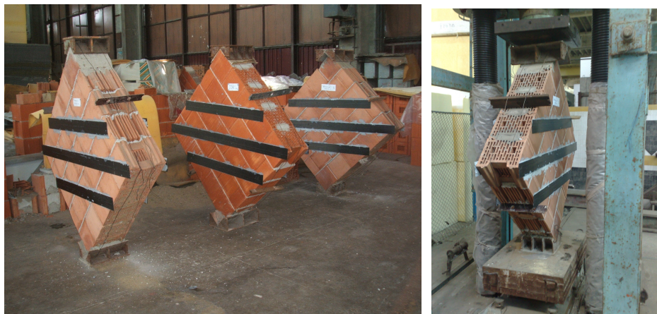
Figure 1. The 3 specimens made of Wienerberger POROTHERM clay blocks after placing Carbon Fibre Plates Sika Carbodur S 1012 (left) and Specimen no. 1 in the testing machine at INCERC (right).
