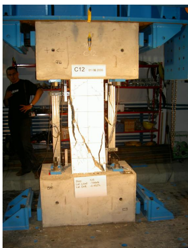
Figure 3 Test on RC columns (original specimen, retrofitted specimen with steel plate and with CF sheet)
