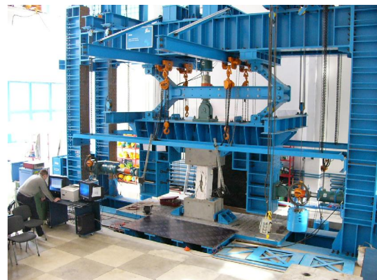
Figure 2 Reaction frame and Column Specimen
