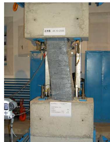
Figure 3 Test on RC columns (original specimen, retrofitted specimen with steel plate and with CF sheet)
