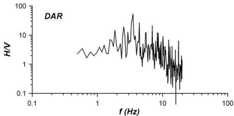
Figure 7. Computed H/V spectral ratio at the DAR station
