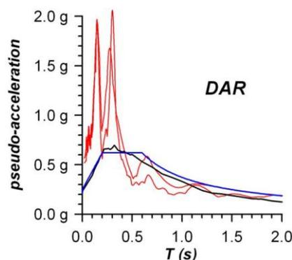
Figure 6. Pseudo acceleration spectra (in red) for the NS and EW components, UHS (in black) specifically computed for the site, and EC-8 horizontal elastic response spectra (in blue), all damped at 5%, for the DAR station
