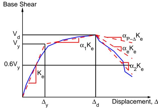
Figure 1. Idealized force-deformation curve in ASCE/SEI 41-06.
