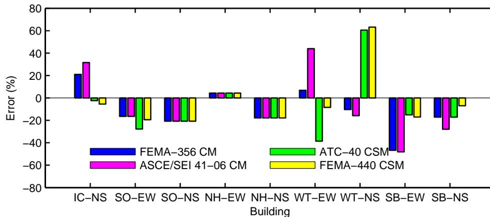
Figure 2. Percent error in peak roof displacements from the FEMA-356 CM, ASCE/SEI 41-06 CM, ATC-40 CSM, and FEMA-440 CSM.
