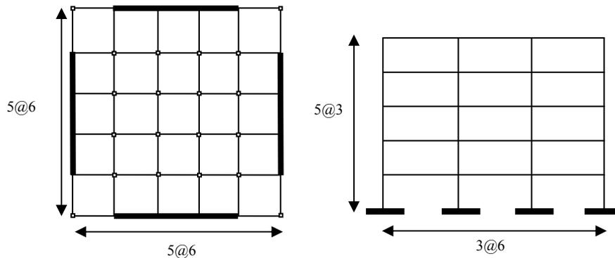
Figure 3 Five-storey steel office building structure
