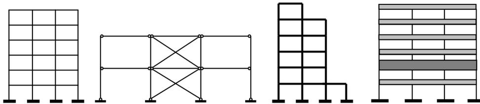
Figure 1 Types of planar steel building frames considered in the HFD seismic design method
