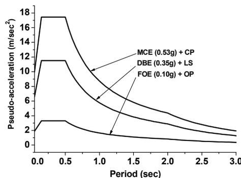
Figure 4 EC8 elastic design spectra
