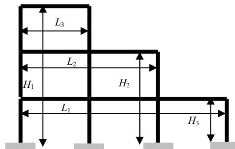
Figure 2 Geometry of frame with setbacks for definition of geometrical irregularity indices
