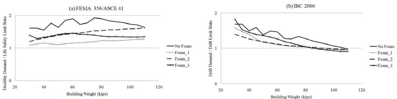
Figure 3.1: One-Story Results for Design Level Earthquake Using FEMA 356/ASCE 41(a) and IBC 2006(b)
