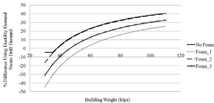
Figure 3.4: Percentage Difference Between Normalized Ductility Demand and Normalized Drift Demand
