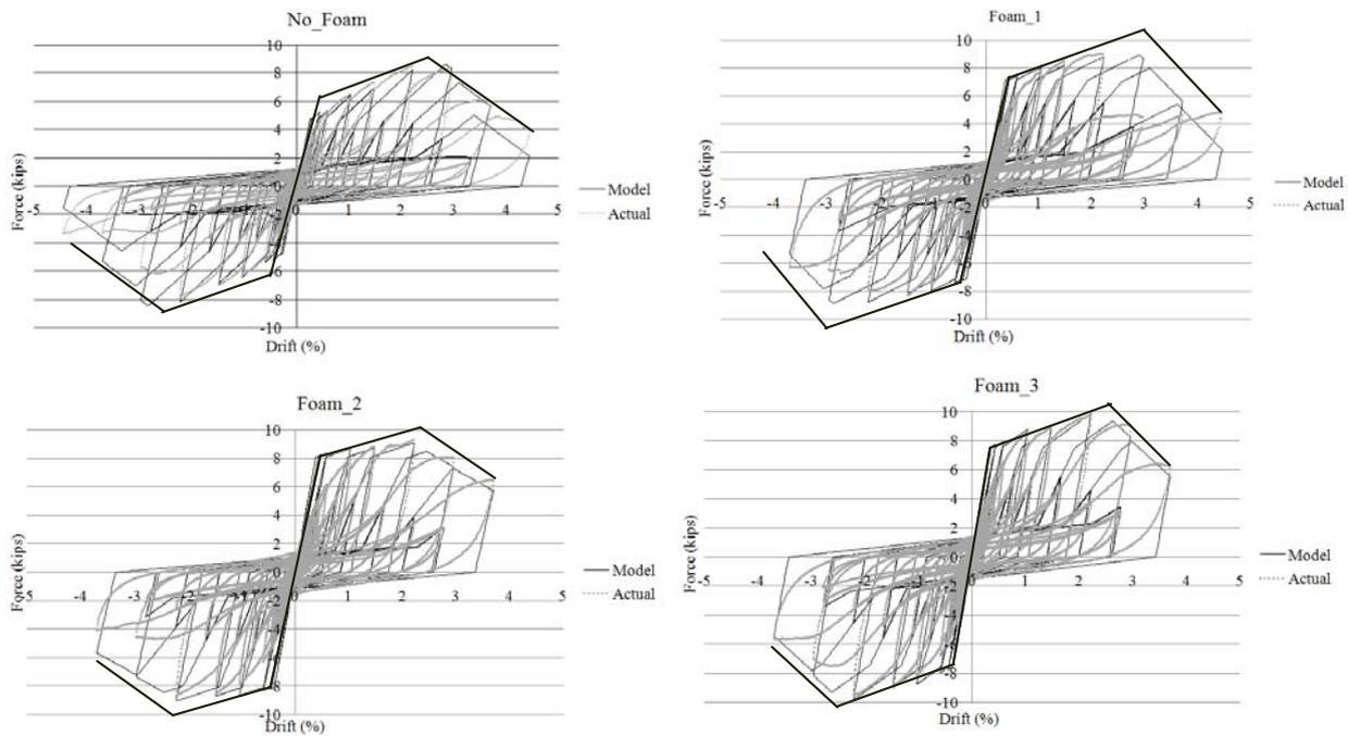
Figure 2.3: Model Calibration with Testing Results and Hysteresis Fit
