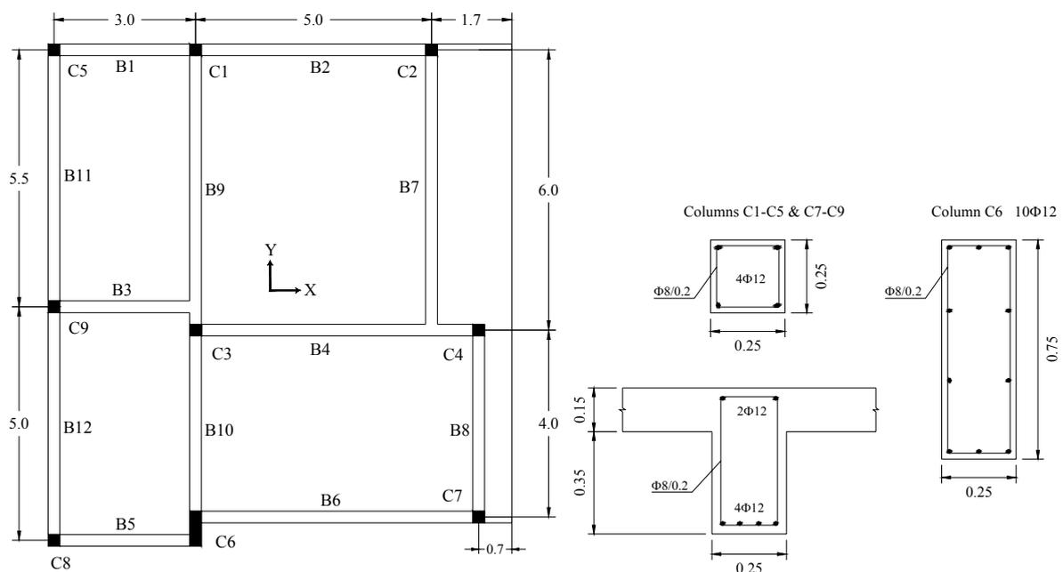
Figure 1 Plan of the test model and drawings of member sections
