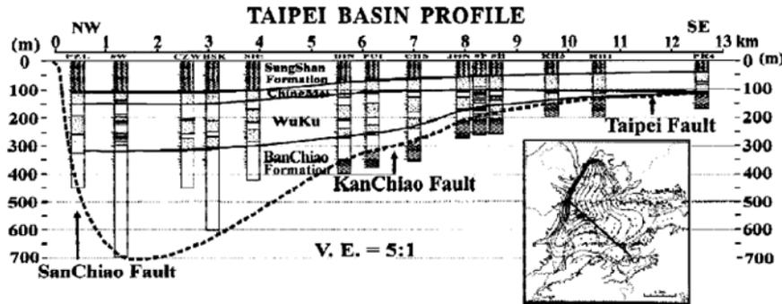
Figure 1 A profile across the Taipei basin perpendicular to the strikes of the faults. (Wang *et al.*, 2004)
