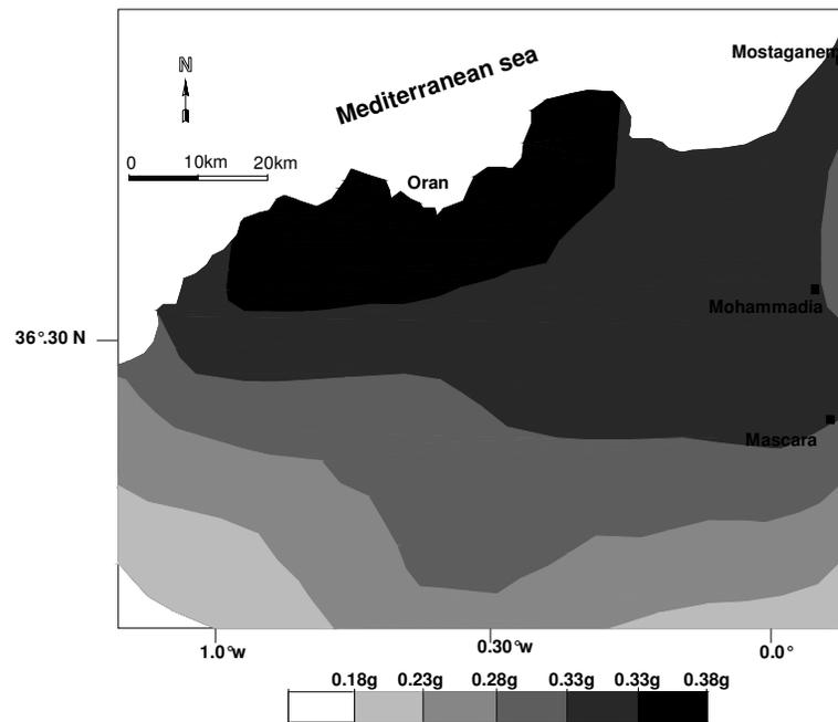
Figure 5 Seismic hazard map of the studied area for a return period of 500 years.
