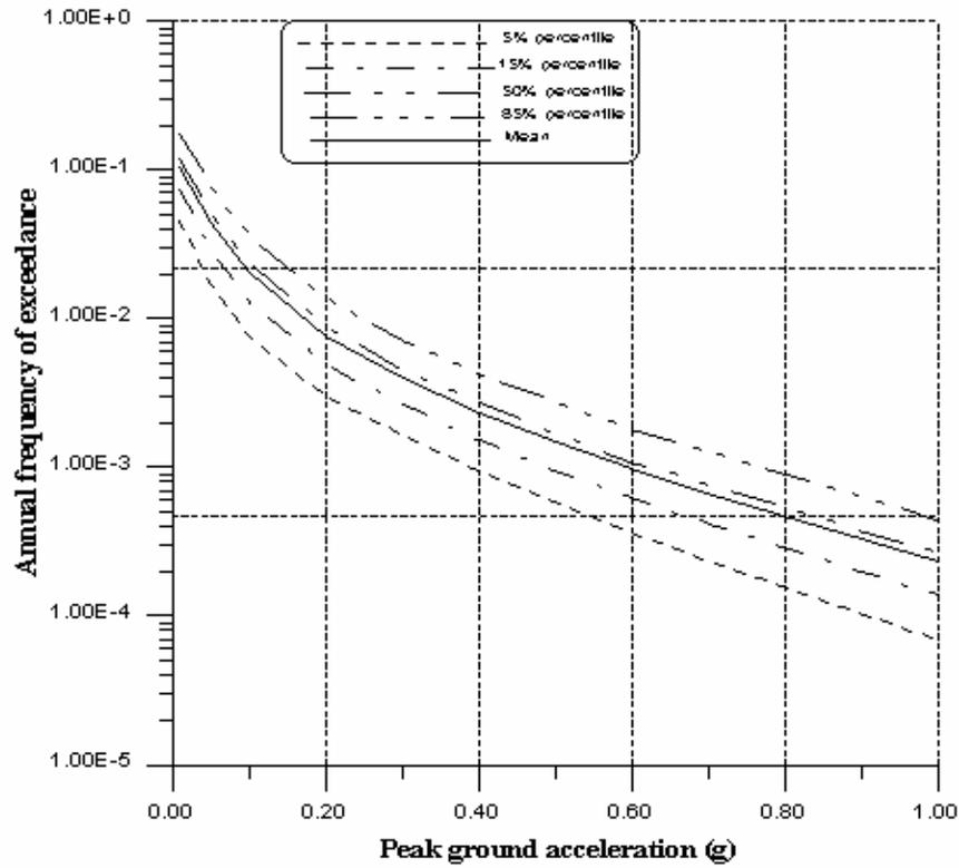
Figure 4 peak ground accelerations versus annual frequencies of exceedance for the Oran site.
