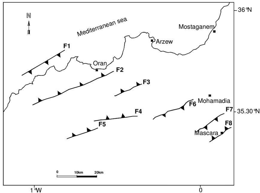
Figure 3 seismic source model of the studied area showing the location and dipping of the identified active faults.
