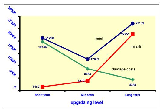
Figure 3. Various curves of retrofit costs and damages costs (in USD) vs upgrading level for main transmission lines in neighborhood No. 28 of Tehran Metropolis for finding the optimum level of upgrading
