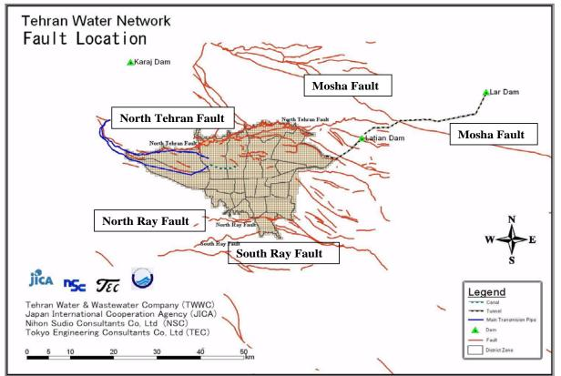
Figuer 1. Tehran water network and seismic faults (JICA 2000)
