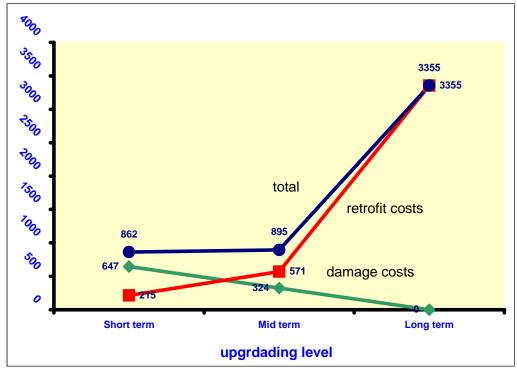
Figure 4. Various curves of retrofit costs and damages costs (in USD) vs upgrading level for main distribution lines in neighborhood No. 28 of Tehran Metropolis for finding the optimum level of upgrading
