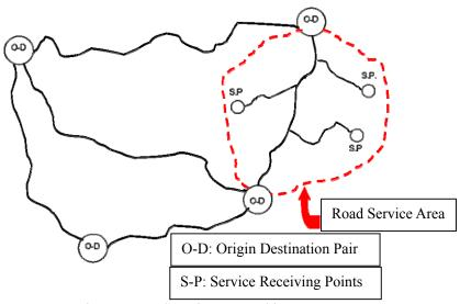
Figure 1. Road service area and its components
