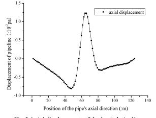
Fig 5 Axial displacement of the buried pipeline
