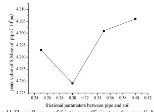
Fig 11 The influence of friction coefficient on the max S, Mise
