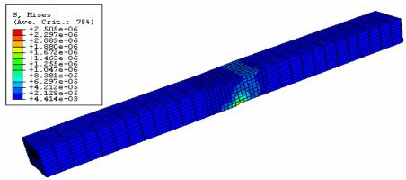
Fig 6 S, Mise of the soil around the pipeline
