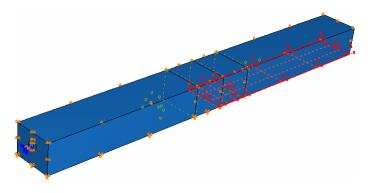
Fig. 1 Interaction model of buried pipeline and soil
