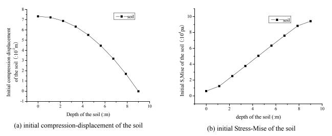
Fig 2 Initial conditions of the soil along the perpendicular direction
