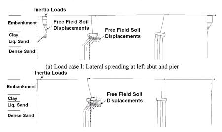
(b) Load case II: Lateral spreading at left pier Figure 4 Bridge deformation under two lateral spreading load cases
