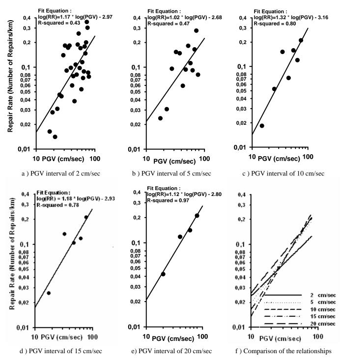
Figure 3 Pipeline damage correlations obtained using PGV contours with various intervals
