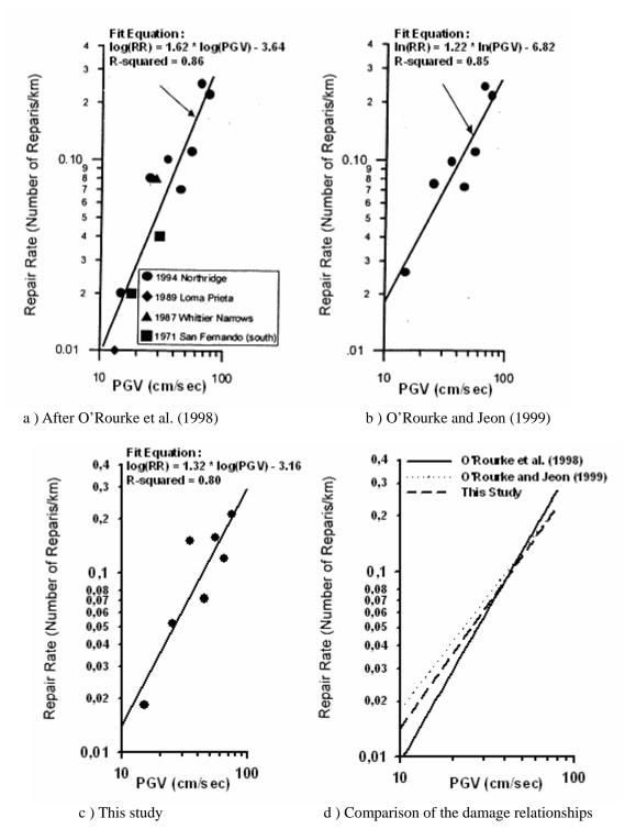
Figure 2 Damage relationships for CI pipelines
