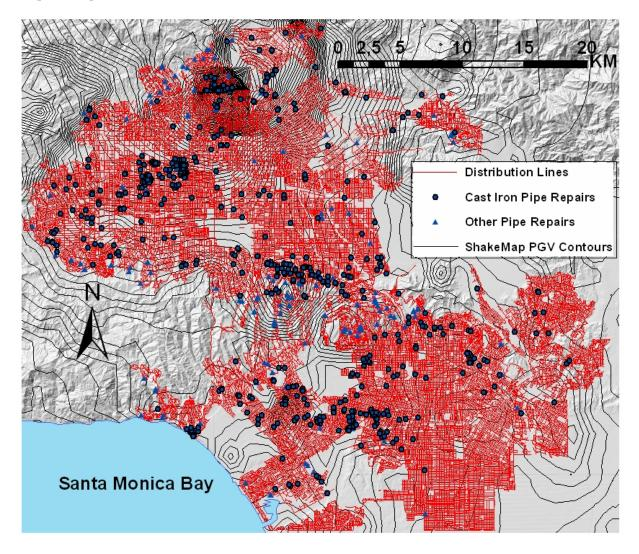
Figure 1 LADWP distribution lines and repairs superimposed on the 1994 Northridge earthquake ShakeMap PGV contours
