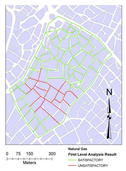
Figure 5 Stage 1 analysis results for the part of the gas pipeline system in Denizli, Turkey
