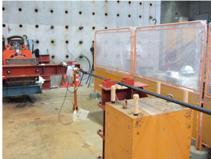
Figure 13 Optical fiber tensile test status
