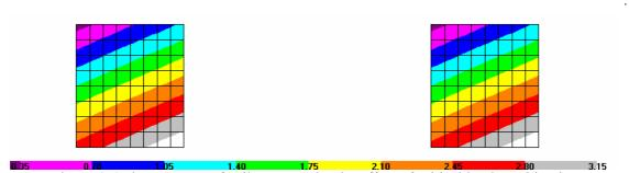
Figure 8.6 The contours of soil stress under the effect of critical load combination
