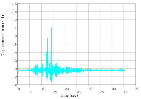
Figure 3 Uplift displacement time history of tank type 22 due to Tabas record
