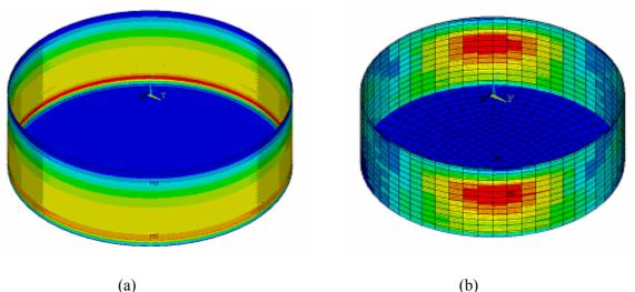
Figure 2 Von-misses stresses of tank shell due to a) hydrostatic forces and b) spectral forces
