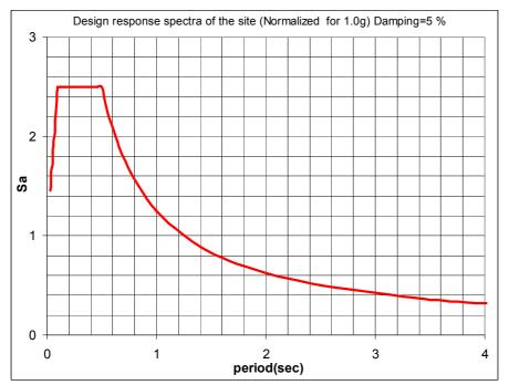
Figure 1 Normalized site-specific response spectra for design earthquake
