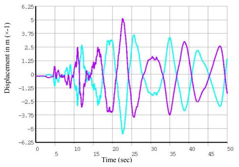
Figure 4 Sloshing displacements time history of tank type 22 due to Tabas record
