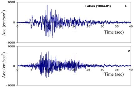
Figure 4 Horizontal (L) and vertical (V) component of Tabas record
