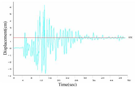
Figure 7 Deck lateral displacement time history of model A subjected to H component of Tabas record with PGA=0.3g.
