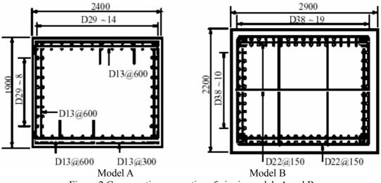
Figure 2 Cross section properties of pier in models A and B
