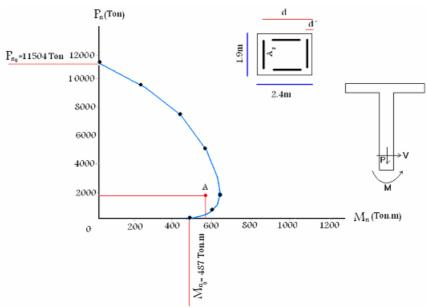
Figure 5 P-M diagram of pier in model A
