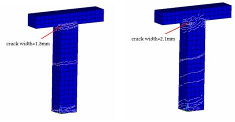
a) H components b) H+V components Figure 9 Crack pattern of model A subjected to a) H components and b) H+V components of Tabas record with PGA=0.5g.
