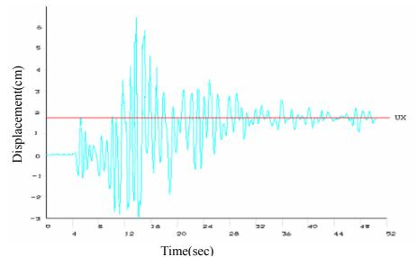
Figure 8 Deck lateral displacement time history of model A subjected to H+V component of Tabas record with PGA=0.3g.
