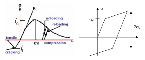
a) Concrete b) Steel reinforcement Figure 3 Nonlinear models for a) Concrete and b) Steel reinforcement
