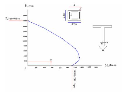
Figure 6 P-M interaction diagram of pier in model B
