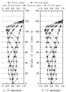
Figure 2 The initial 5 vibration modes of SZK122
