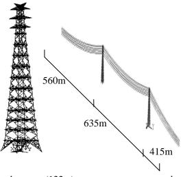
*a* Single tower (122*m*) *b* system Figure 1 The finite element model of 220 SZK combo steel tube transmission lines towers
