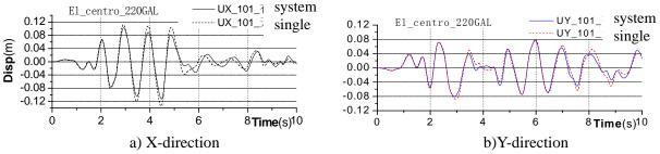
Figure 3 X, Y-directional displacement ratio of A4 tower head's 101node between single tower and systems
