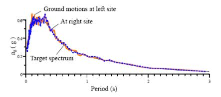
Figure 2. Australian design spectrum and response spectra of the simulated intermediately correlated ground acceleration with the apparent wave velocity of 500 m/s
