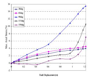
Figure 6. Variation of maximum axial strain with fault displacement
