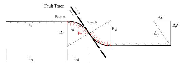
Figure 1. Soil-pipeline model using Kennedy's approach
