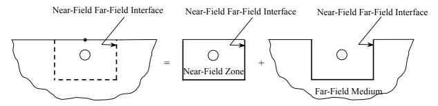
Figure 3. New hybrid model for soil pipe segment (Halabian et al. (2008))
