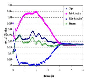
Figure 8. Variations of axial strains along the pipe for crossing angle 65<sup>0</sup>
