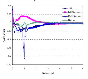
Figure 9. Variations of axial strains along the pipe for crossing angle 110<sup>0</sup>
