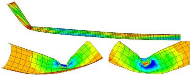
Figure 5. Local deformations of the pipe subject to fault movement
