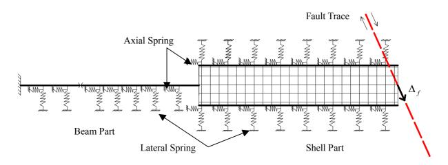
Figure 2. Soil-pipeline FEM model
