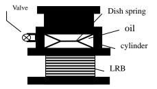
Figure 1 three dimension isolated device
