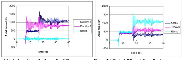
Figure 6 Variation of transfer forces for different structural ductility levels at level 1 of the structure
