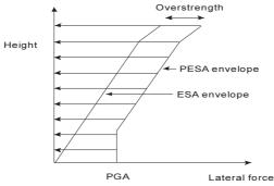
Figure 2 Static forces for ESA and pESA envelopes
