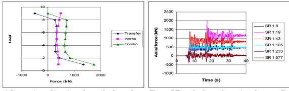
Figure 4 Comparison of inertia and transfer forces for SR1:43 and structural ductility of 3
