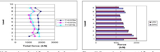
Figure 10 Comparison of total floor forces for frame to wall structures with the same stiffness ratios but different fundamental time periods
